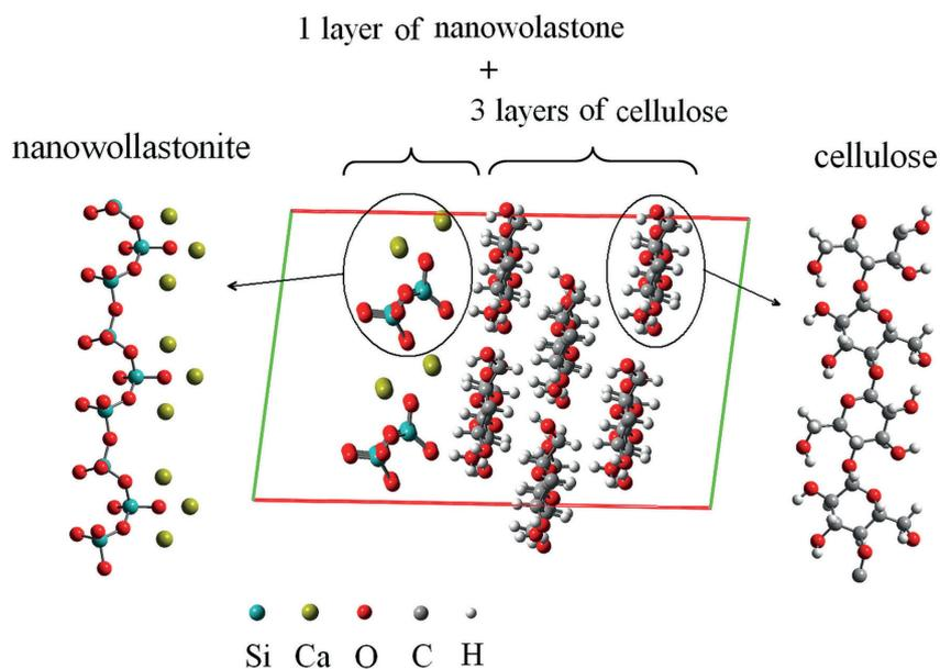
**Figure 4** - Schematic representation of bond formation between Calcium atoms of NW and Oxygen atoms of cell-wall cellulose chains (Taghiyari et al. 2016).
