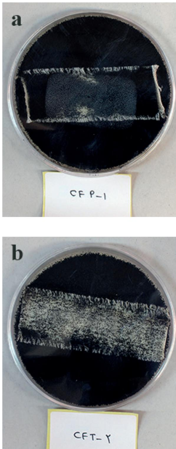
**Figure 2** - Visual observation of the control (a) and NW-impregnated (b) specimens after three months of exposure to *A. nigr* in Petri dish.
