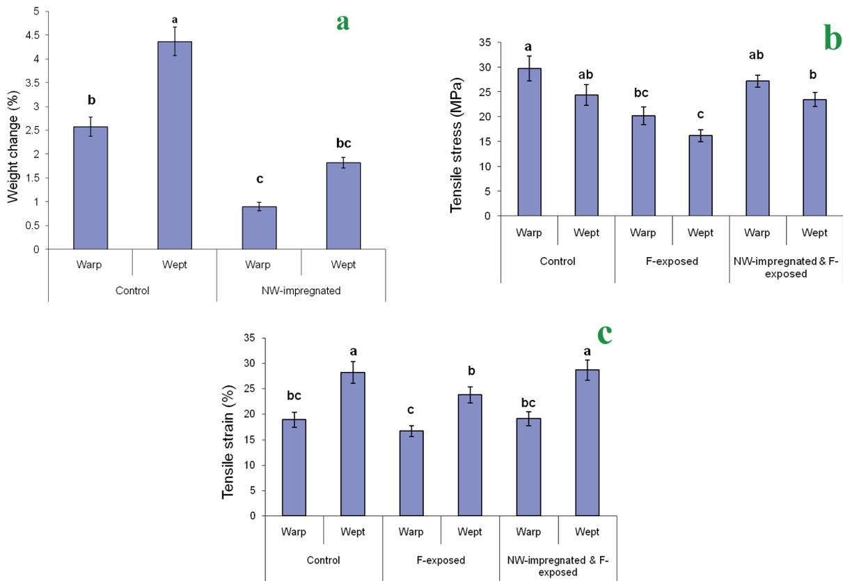
**Figure 3** - Weight changes (a), tensile stress (b), and tensile stress (c) values in the control and NW-impregnated cotton cloth specimens in warp and weft directions, exposed to *A. nigra* for three months (capital letters on each column represent Duncan's groupings).
