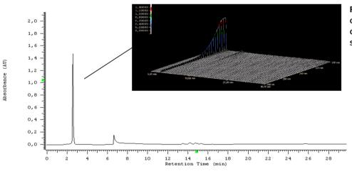
**Figure 3.** Chromatogram of 1E-1/AF using RP chromatography, UV spectrum (DAD A<sub>200</sub> - A<sub>280</sub>).
