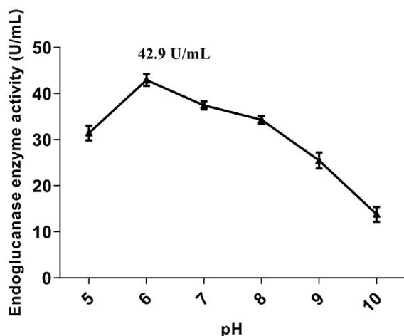
**Figure 7.** The effect of initial pH on the endoglucanase enzyme activity. Culture conditions: MPP concentration 50 g/L, 2 g/L yeast extract, Temperature 40°C, and incubation time 48 h.
