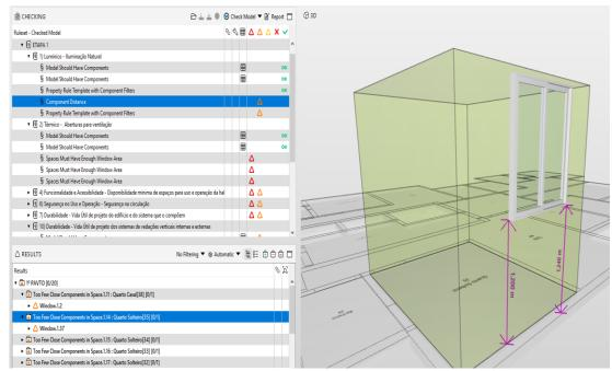
Figure 5 - Nonconformity concerning the window-sill height in the BIM model
