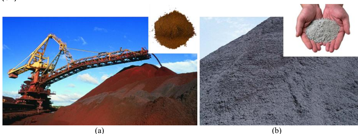
Figure 1 - Illustrative images of the materials used: (a) iron ore tailings (IOT) and (b) gneiss powder (GN)
