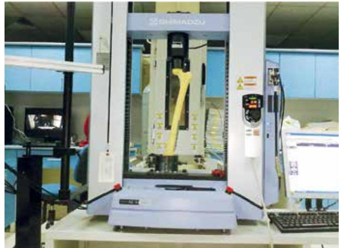
Figure 1. The experimental setup with one specimen is shown. The specimen is positioned anatomically on the uniaxial testing machine.
