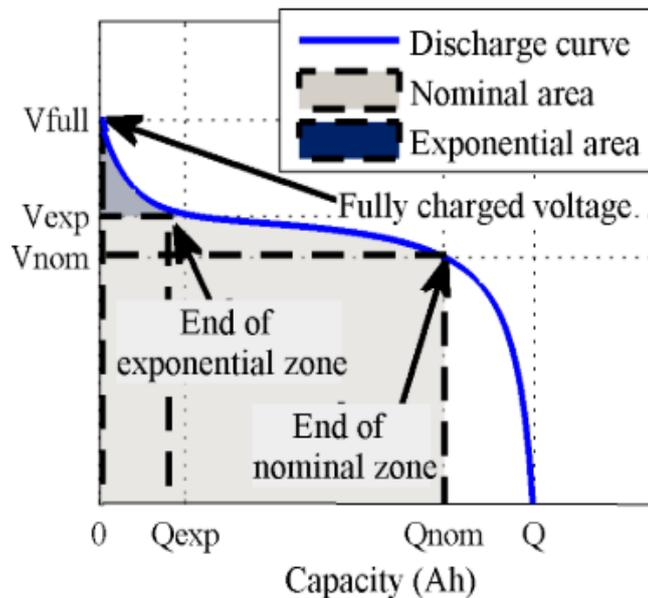
**Figure 1.** Typical discharge curve for li-ion battery.
