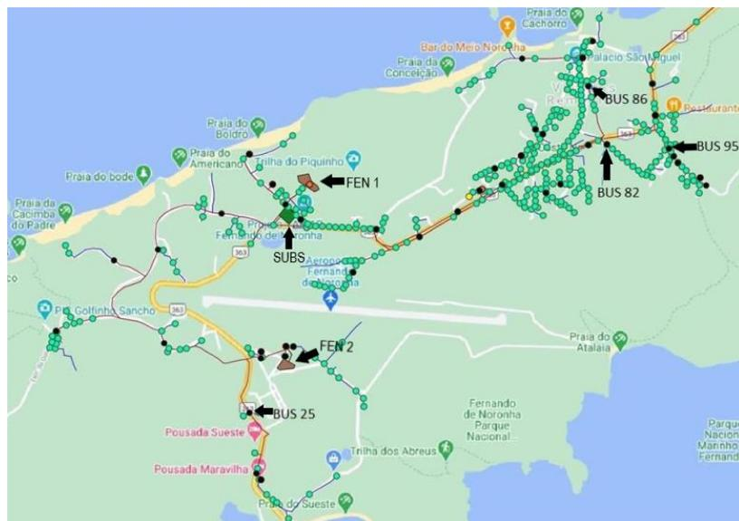
**Figure 7.** Location of the Buses with EV Chargers, the substation (SUBS), and the solar generation power plants (FEN 1 and FEN 2).
