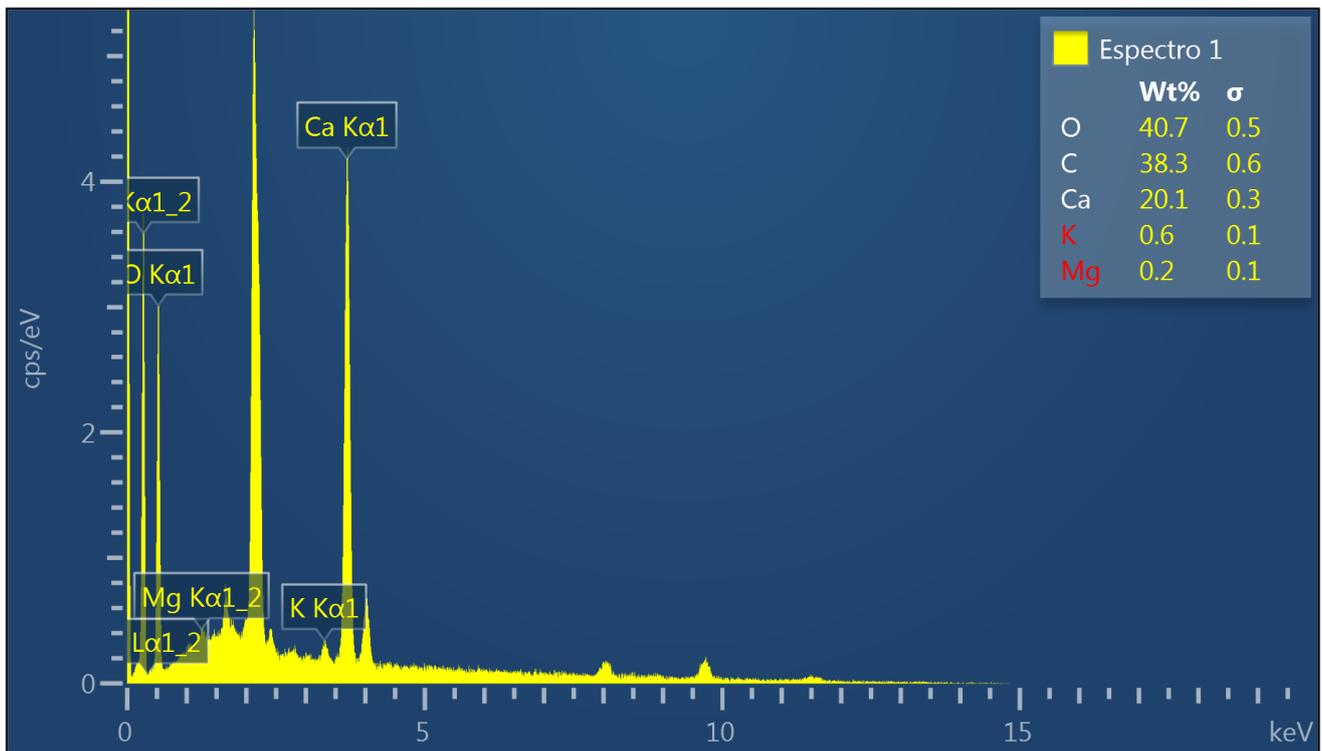
**Figure 3.** Energy-dispersive X-ray Spectroscopy (EDS) spectrum of prismatic crystal from *Acmeella bellidioides*.
