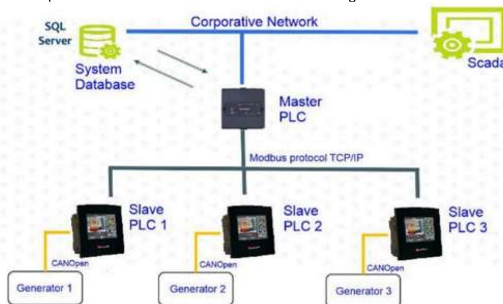
**Figure 1.** Network topology and main equipment and devices.
