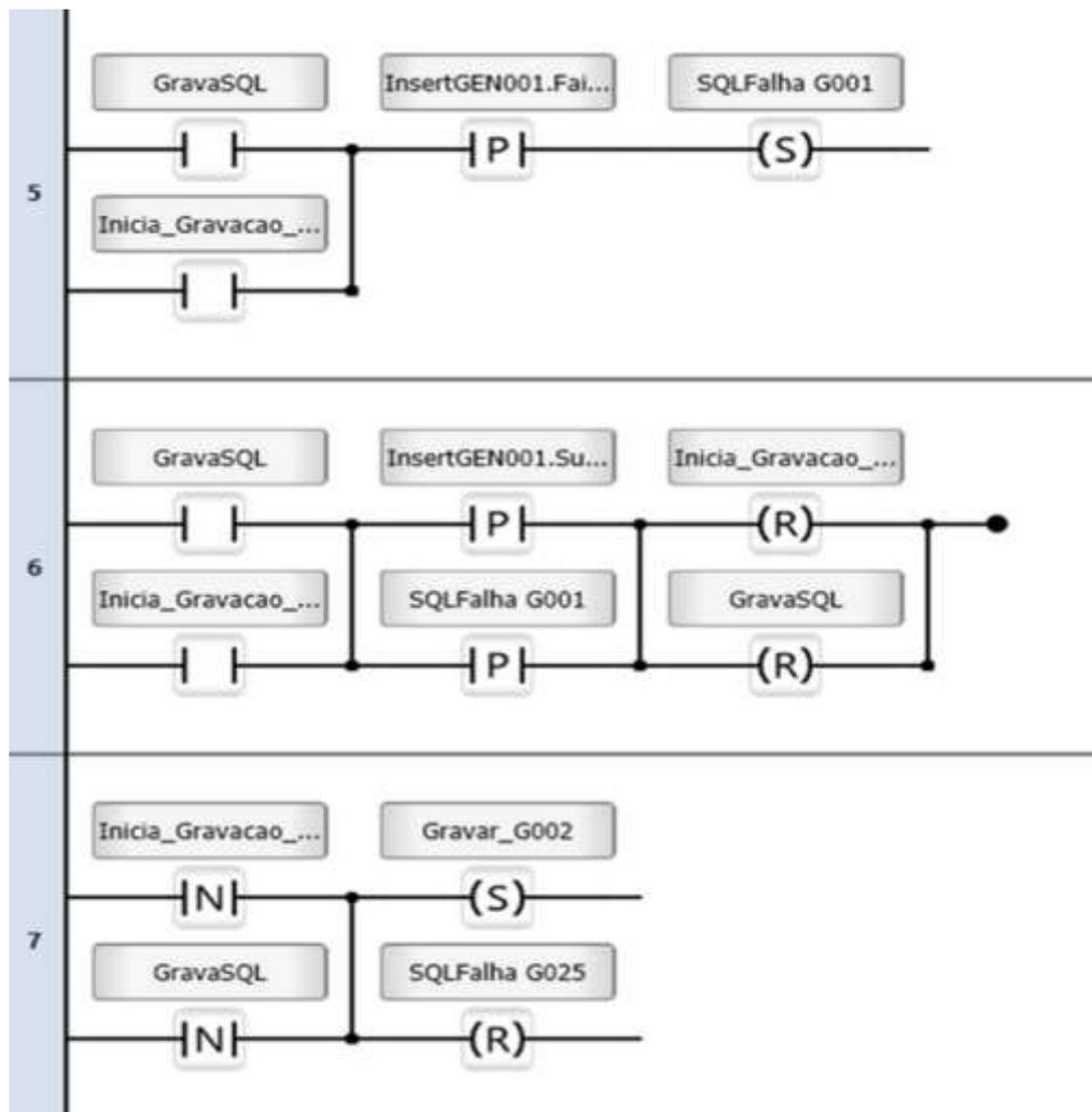
**Figure 5.** Process of checking for errors in SQL execution on the database server.
