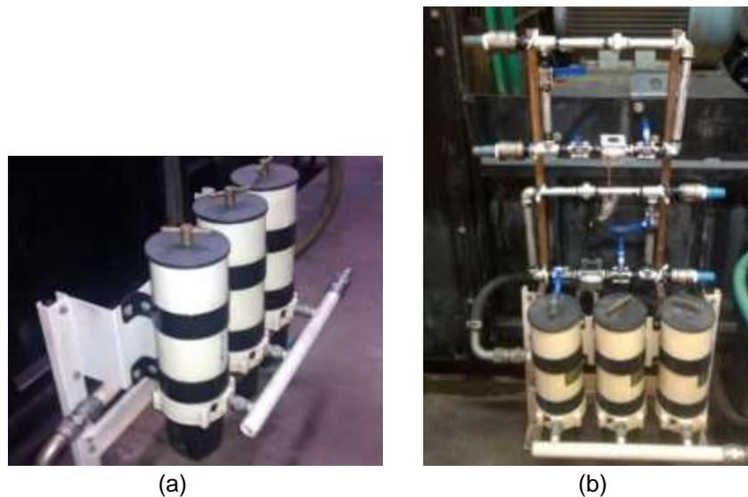
**Figure 2.** PIUSI fuel meter placement – entrance side: (a) before installation, and (b) after the installation.
