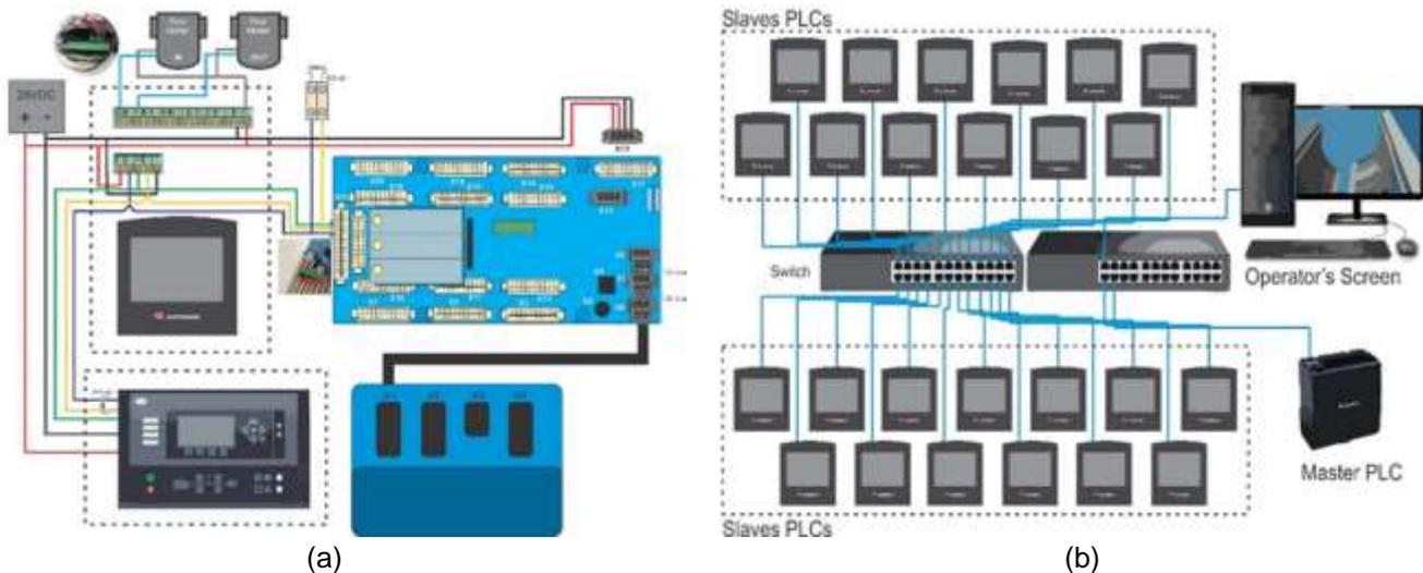
**Figure 7.** Topology: (a) integration between slave PLCs, and (b) final network installed at the Palmeiras de Goias Thermal Power Plant.
