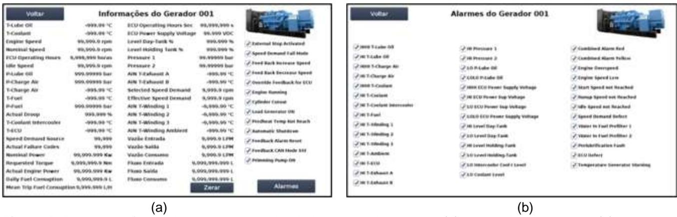
**Figure 6.** Examples of operator's screens related to the generator unit #1: (a) parameter screen and (b) alarm screen.
