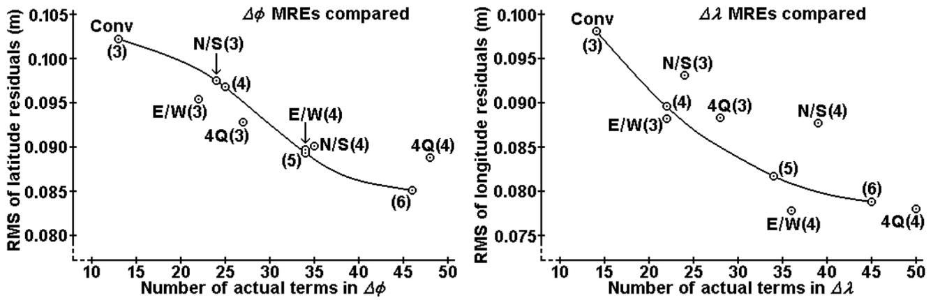
Figure 3: Partitioned-vs-conventional accuracy comparison for D48→D96 datum shift.
