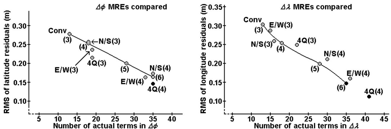
**Figure 4:** Partitioned-vs-conventional accuracy comparison for AGD84→GDA94 datum shift
