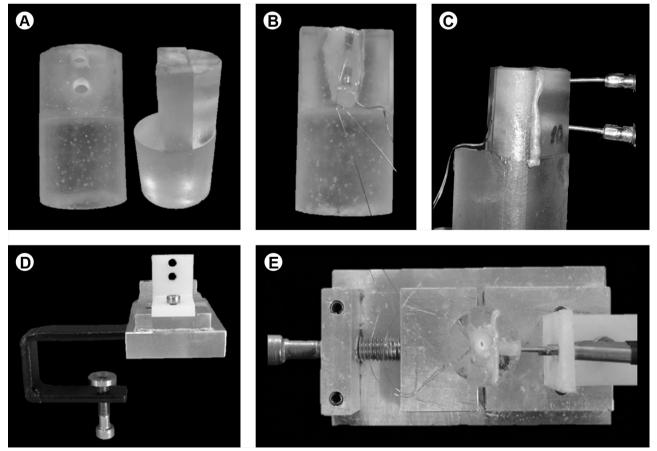
Figure 1. Experimental device used for temperature rise and strain measurement. A: Cylinder for strain gage and thermocouple attachment. B: Cylinder sustaining apparatus. C: Cervical and apical strain gages fixed in the distal root surface region. D: Lateral polytetrafluoroethylene support to fixe the cervical and apical J-thermocouples on mesial root surface region. E: Experimental device with sample connected to the strain gauges and thermocouples.
