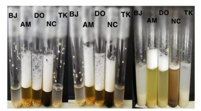
Figure 1. Foam column in quinoa materials for each Afrosymetric method. (A) Standard Afrosymetric Method (MAE); (B) modified afrosymetric method (MAM); (C) Rapid Afrosymetric Method (MAR).
