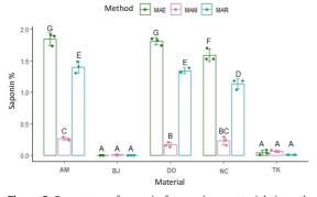
**Figure 2.** Percentage of saponin from quinoa materials in each Afrosymetric method. Different letters indicate significant differences according to the Fisher's mean comparison test (LSD) ( $p \le 0.05$ ). Vertical bars indicate standard error (n=3).
