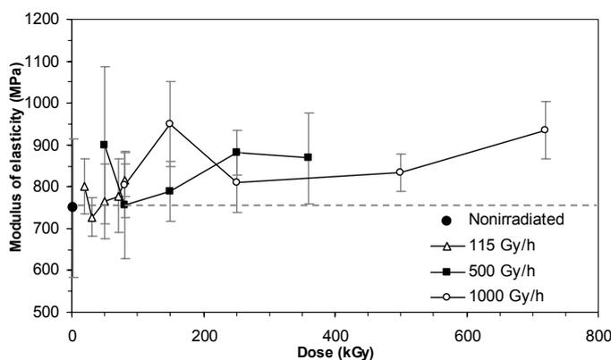
**Figure 3:** Modulus of elasticity of irradiated samples from compression tests as a function of dose and dose rate. Error bars indicate the 95% confidence interval.
