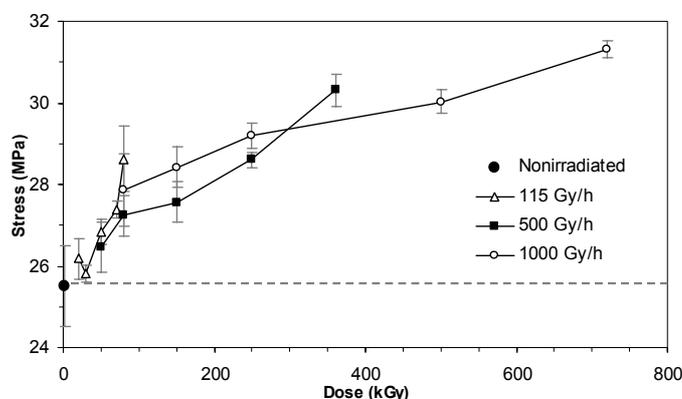
**Figure 1:** 5% offset yield stress of irradiated samples from compression tests as a function of dose and dose rate. Error bars indicate the 95% confidence interval.
