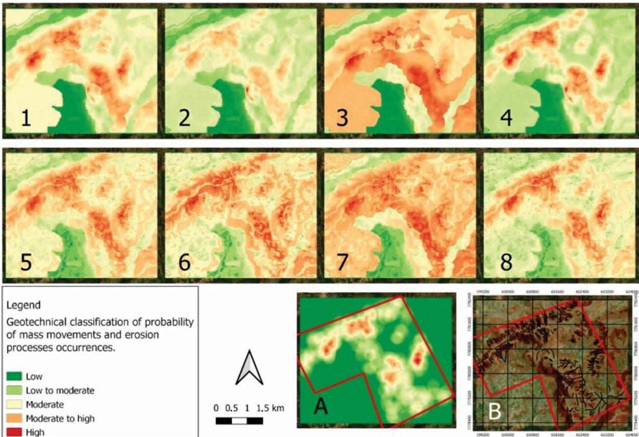
**Figure 8.** Scenarios of geotechnical analysis based on slope, lithology, and lineament density. Numbers 1–8 correspond to the eight scenarios generated. Map A: line density map where red represents the highest line density values and green the lowest, while yellow are the moderate density areas. Map B represents slope together with traced lineaments (in black), where red is the highest slope and green the lowest.
