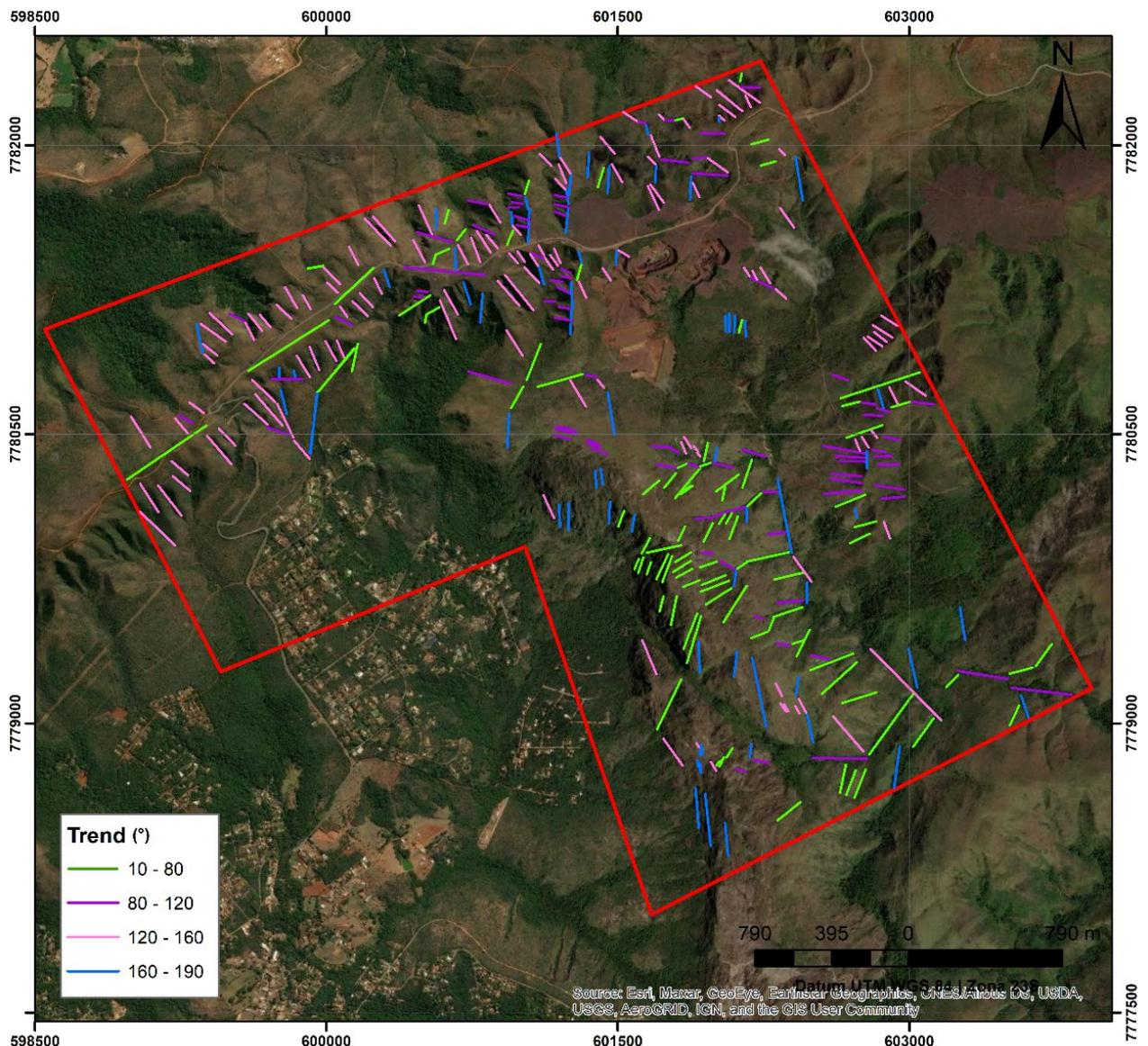
**Figure 6.** Lineaments traced remotely and divided in sets. Set 1 ( $10^{\circ}$ – $80^{\circ}$ ) in green, Set 2 ( $80^{\circ}$ – $120^{\circ}$ ) in purple, Set 3 ( $120^{\circ}$ – $160^{\circ}$ ) in pink, and Set 4 ( $160^{\circ}$ – $190^{\circ}$ ) in blue. Satellite image from ESRI (2021).
