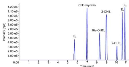
**Figure 4.** Total ion flow chart. E<sub>1</sub>: estrone; E<sub>2</sub>: estradiol; E<sub>3</sub>: estril; 2-OHE<sub>1</sub>: 2-hydroxyestrone; 2-OHE<sub>2</sub>: 2-hydroxyestradiol; 16a-OHE<sub>1</sub>: 16a-hydroxyestrone.
