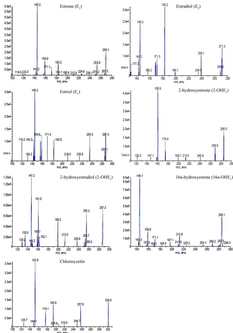
**Figure 3.** Product mass spectrum of EMs and internal standards. E<sub>1</sub>: estrone; E<sub>2</sub>: estradiol; E<sub>3</sub>: estriol; 2-OHE<sub>1</sub>: 2-hydroxyestrone; 2-OHE<sub>2</sub>: 2-hydroxyestradiol; 16a-OHE<sub>1</sub>: 16a-hydroxyestrone; chlormycetin.
