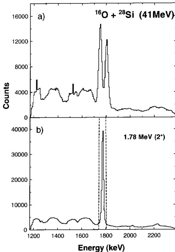
Figure 3. A region of a  $\gamma$ -ray spectrum; a) before Doppler shift correction and b) after Doppler Shift correction. Panel b) includes the gating condition to obtain the events in coincidence with the 1.78 MeV  $\gamma$ -ray transition deexciting the  $2^+$  excited level in  $^{28}\text{Si}$ .
