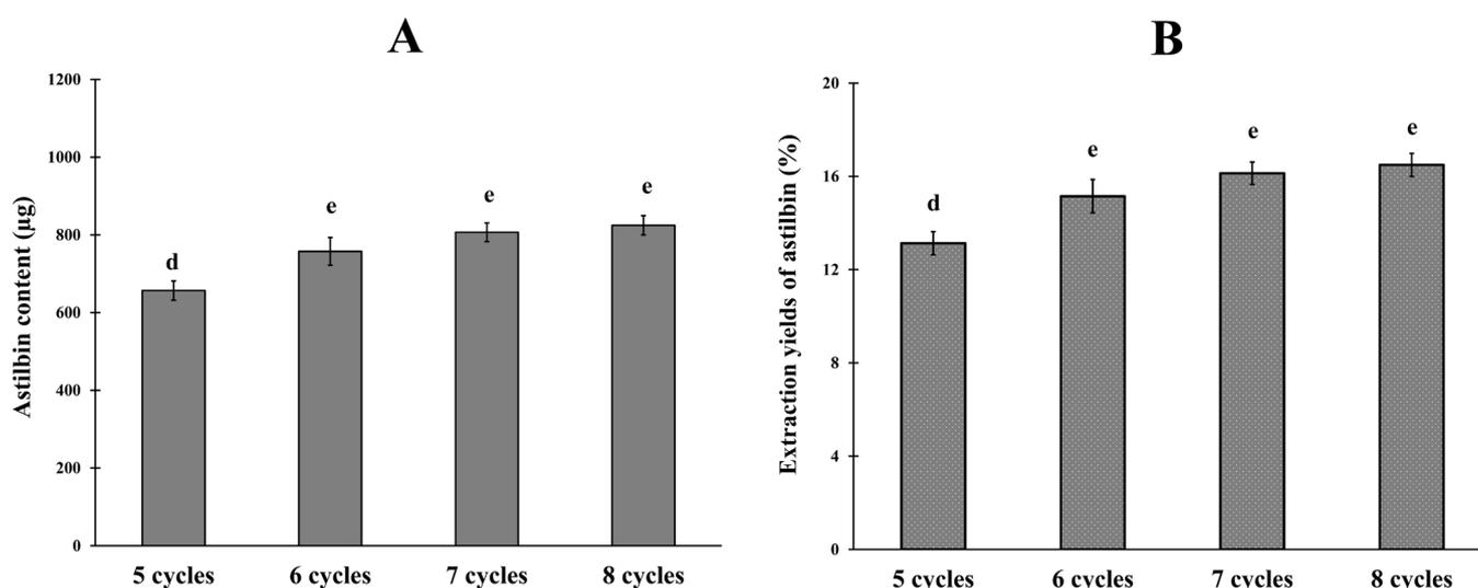
**FIGURE 6** - (A) Astilbin content and (B) extraction yields of astilbin using 450 W of microwave power in water:methanol (40:60) solvent using a different number of microwave-assisted extraction cycles. The extraction yields of astilbin were calculated as dry powder of *L. strychnifolium* stems. <sup>d</sup>significantly different ( $p < 0.05$ ). <sup>e</sup>significantly different ( $p > 0.05$ ).
