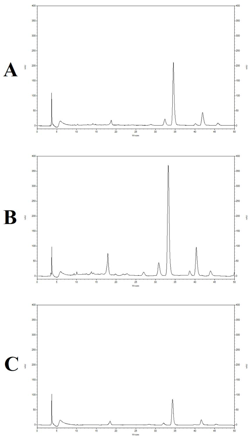
**FIGURE 3** - HPLC chromatogram of astilbin using 300 W of microwave power and six cycles of microwave-assisted extraction in different solvents: (A) ethanol, (B) water:methanol (40:60), and (C) ethyl acetate.
