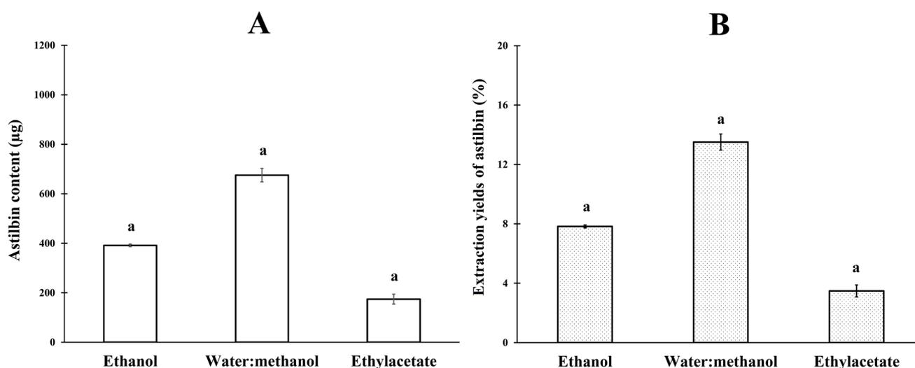
**FIGURE 4** - (A) Astilbin content and (B) extraction yields of astilbin using 300 W of microwave power level and six cycles of microwave-assisted extraction in different solvents: ethanol, water:methanol (40:60), and ethyl acetate. The extraction yields of astilbin were calculated as dry powder of *L. strychnifolium* stems. <sup>a</sup>significantly different ( $p < 0.05$ ).
