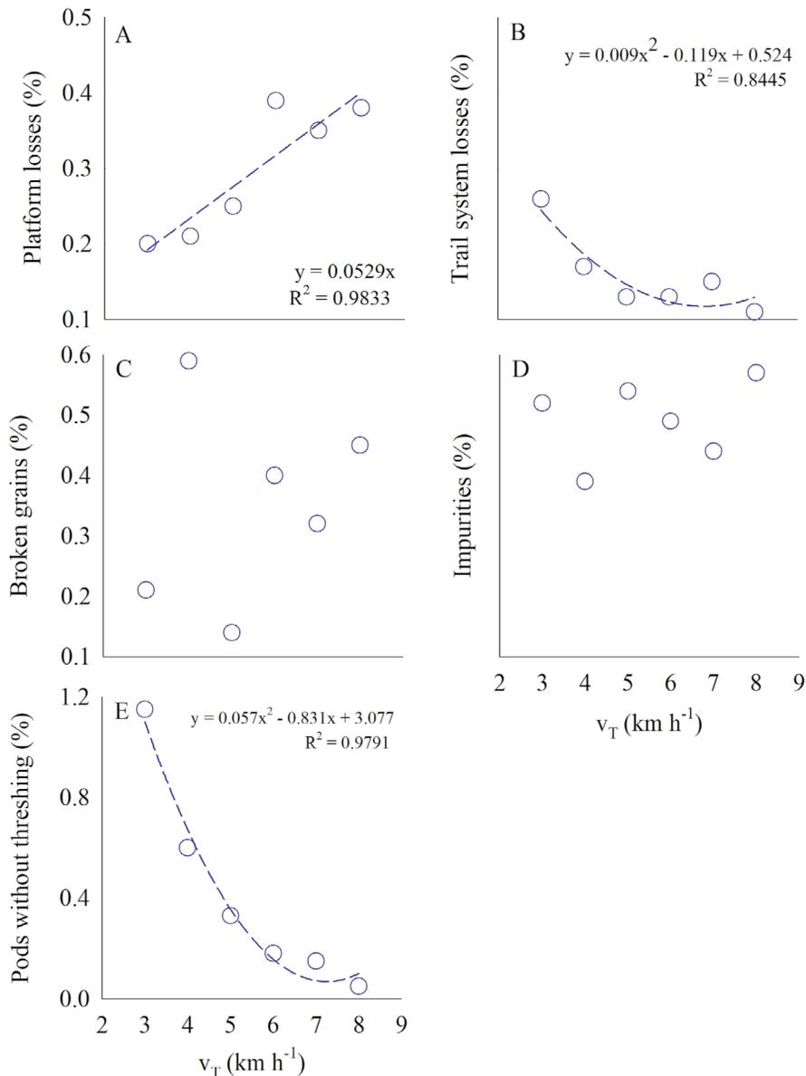
**Figure 3:** Regression analysis for the isolated target velocity ( $v_T$ ) factors in the harvesting performance parameters: (A) platform losses; (B) trail system losses; (C) broken grains; (D) impurities; and (E) pods without threshing.
