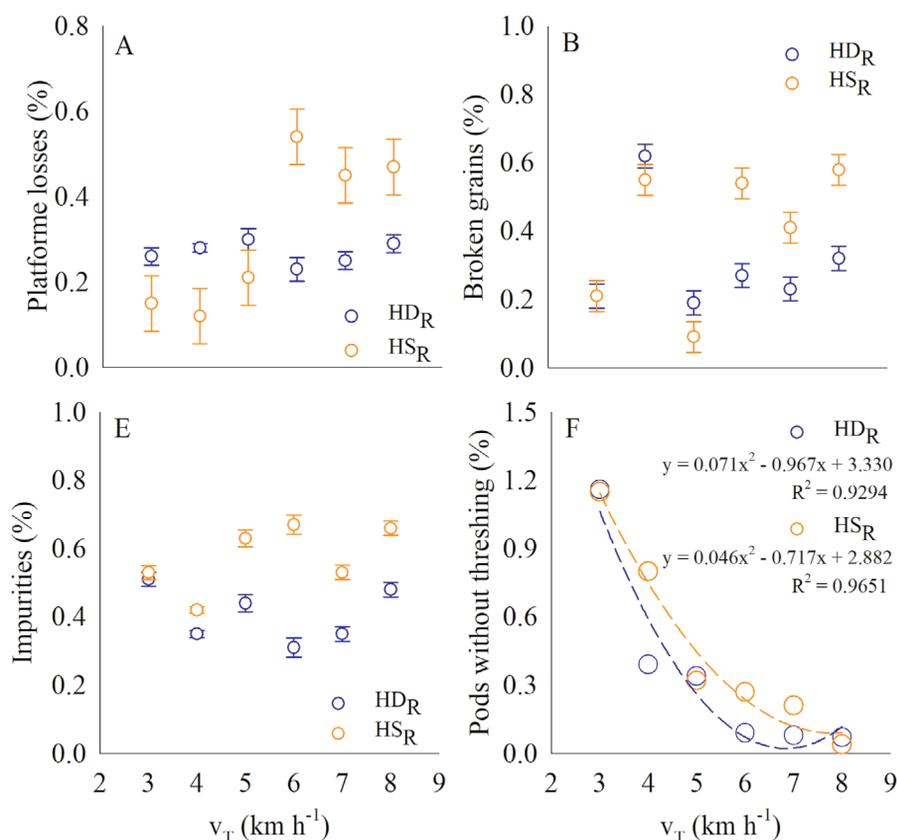
**Figure 4:** Regression analysis of the interaction harvesters ( $H_{SR}$  and  $H_{DR}$ ) and target velocity ( $v_T$ ) in the harvesting performance parameters: (A) platform losses; (B) broken grains; (C) impurities; and (D) pods without threshing.
