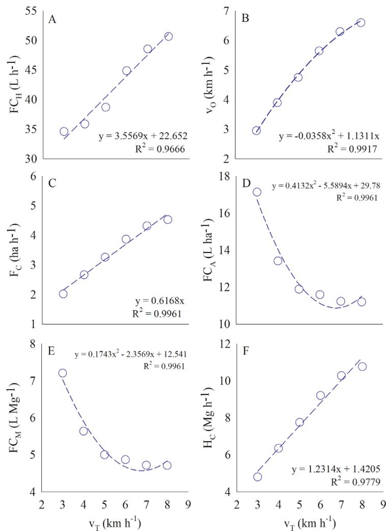
**Figure 1:** Regression analysis for the isolated target velocity ( $v_T$ ) factor in the parameters: (A) hourly fuel consumption ( $FC_H$ ); (B) operational velocity ( $v_o$ ); (C) operational field capacity ( $F_C$ ); (D) fuel consumption per worked area ( $FC_A$ ); (E) fuel consumption per harvested mass ( $FC_M$ ); and, (F) harvest handling capacity ( $H_C$ ).
