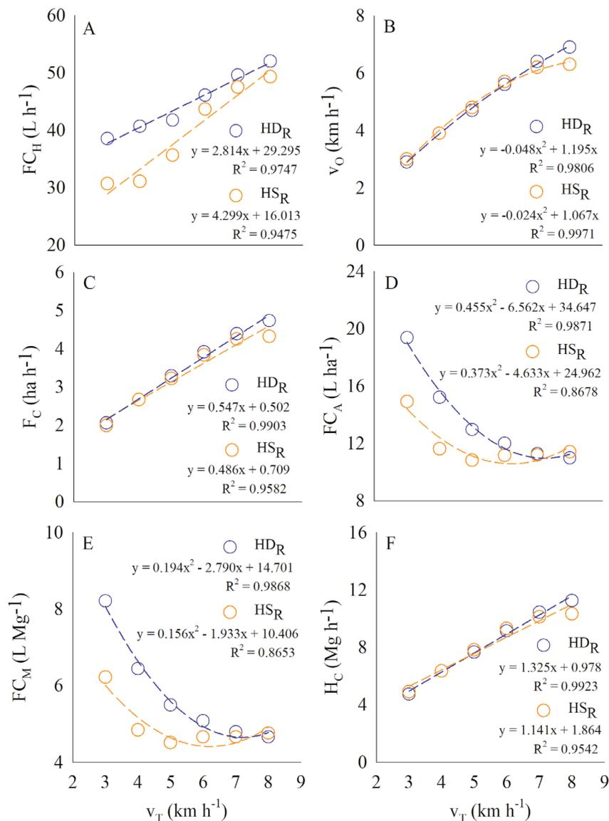
**Figure 2:** Regression analysis of the interaction harvesters (H<sub>SR</sub> and H<sub>DR</sub>) and target velocity (v<sub>T</sub>) in the parameters: (A) hourly fuel consumption (FC<sub>H</sub>); (B) operational velocity (v<sub>O</sub>); (C) operational field capacity (F<sub>C</sub>); (D) fuel consumption per worked area (FC<sub>A</sub>); (E) fuel consumption per harvested mass (FC<sub>M</sub>); and, (F) harvest handling capacity (H<sub>C</sub>).
