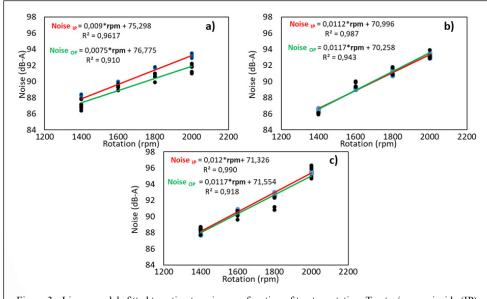
Figure 3 - Linear models fitted to estimate noise as a function of tractor rotation. Tractor/mower inside (IP) and outside (OP) the coffee plantation (a); Tractor/brush inside (IP) and outside (OP) the coffee plantation (b); Tractor/atomizer inside (IP) and outside (OP) the coffee plantation (c).
