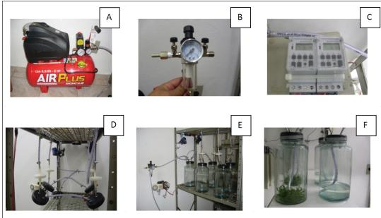
Figure 1 - Air compressor (A), pressure valve (B), temporizer (C), vessels and filters (D), general aspect of the equipment (E), plants cultivated in temporary immersion bioreactor (F). Source: Author's preparing
