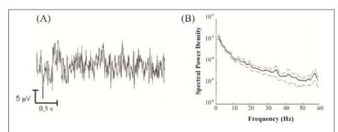
Figure 3 - Pattern of the electrical signal recorded by non-invasive electrodes. (A) EEG signal of 3 seconds; (B) Spectral power density for these stretched under the control condition. Spectrum was calculated using the Welch method with an overlay of 50%. The result shown has a confidence interval of 95% (central line).
