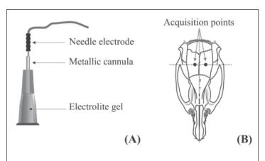
Figure 1 - Representation of the interface to capture electrical brain signals of rats by a non-invasive method for the EEG. (A) Electrode developed from the junction of a guide tube attached to a needle electrode. (B) The system has been fixed to the surface of the skin of the head of the experimental animal.
