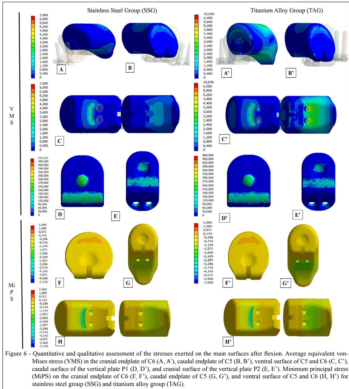
prosthesis may have a stronger correlation with the average forces acting on the bone (VMS) than with only the compressive stresses (MiPs).
