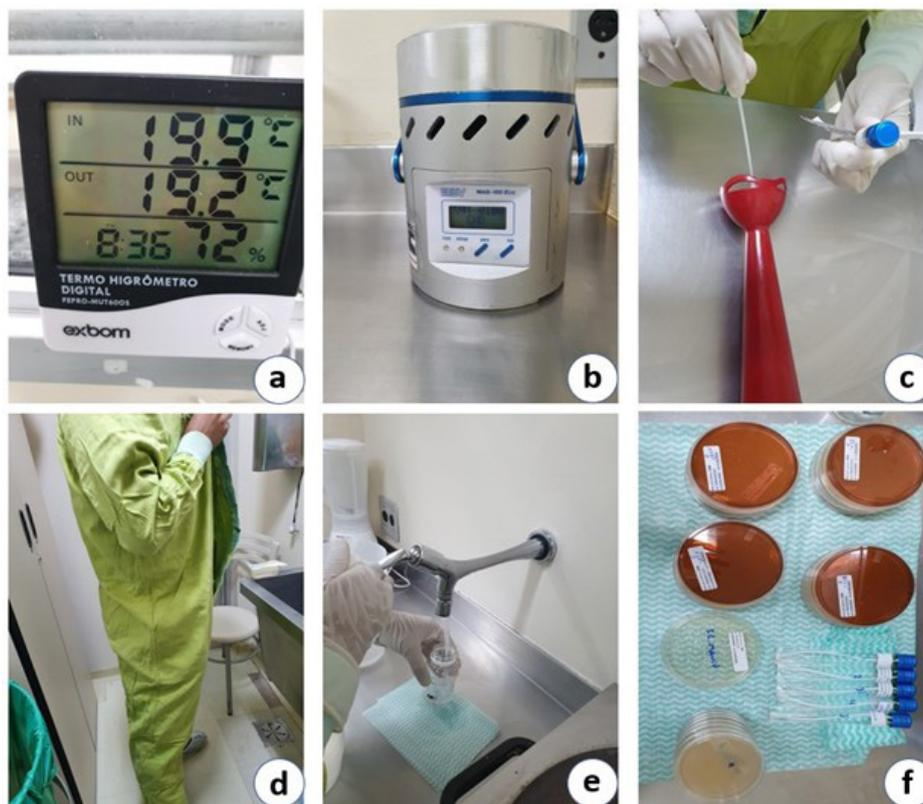
**Figure 2.** Images from the photographic report, refer to the mitigating actions of risks. Thermohygrometer for checking temperature and humidity (a), impactor for analysis of fungi and bacteria from the air (b), mixer Swab (c), the attire of workers' (d), water analysis (e), Swab and wheel of equipment and workers' hands (f).
