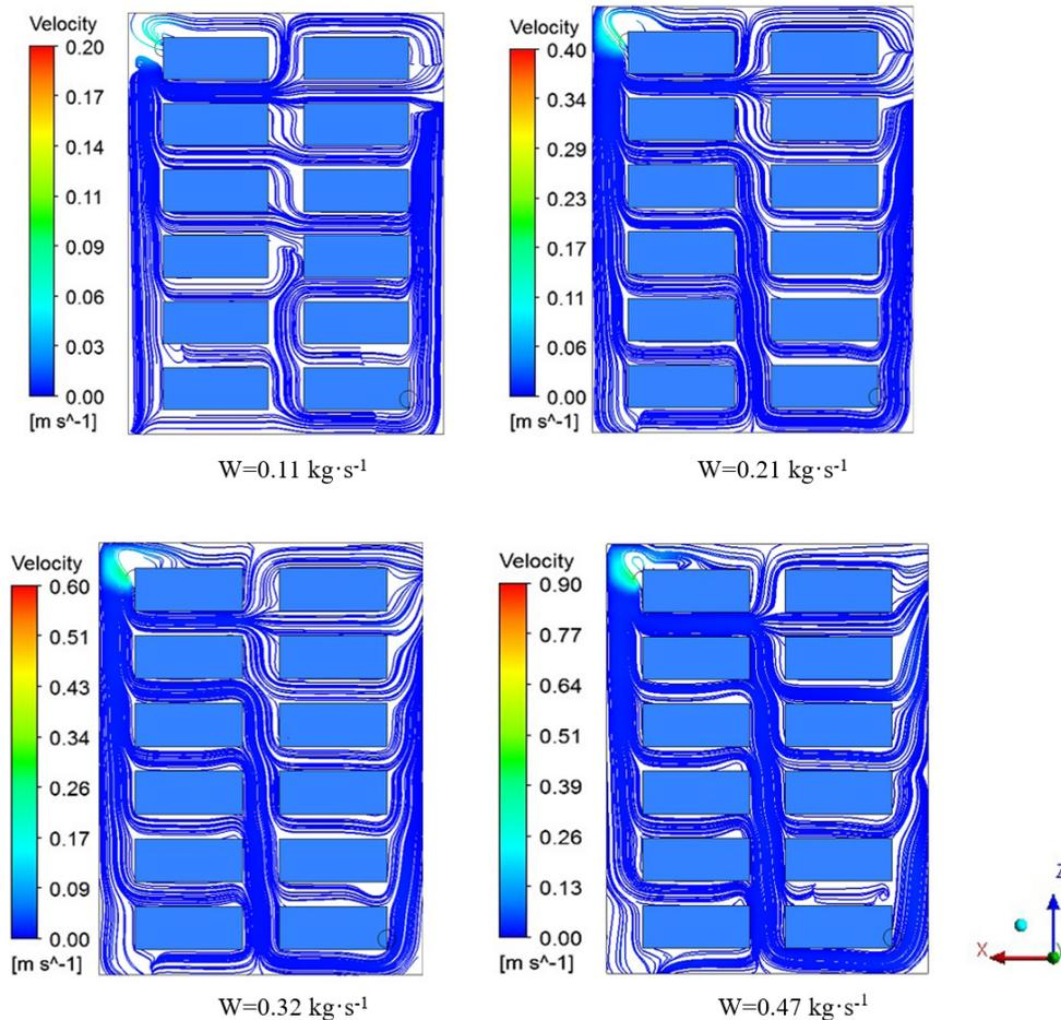
**Figure 2.** Velocity streamline distributions (X-Z plane, Y = 225 mm).
