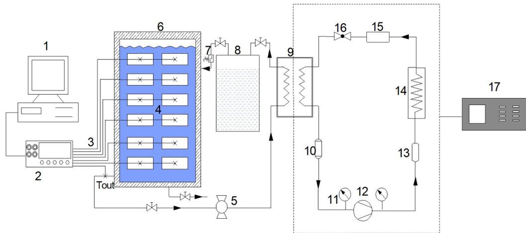
**Figure 1.** Schematic of the experimental setup. 1. Computer; 2. Data acquisition system; 3. Thermocouple extension wire; 4. Samples; 5. Circulation pump; 6. Freezing tank; 7. Ultrasonic flow-meter; 8. Refrigerant liquid storage tank; 9. Evaporator; 10. Gas-liquid separator; 11. Pressure gauge; 12. Compressor; 13. Oil separator; 14. Condenser; 15. Dry filter; 16. Evaporator; 17. Control panel.
