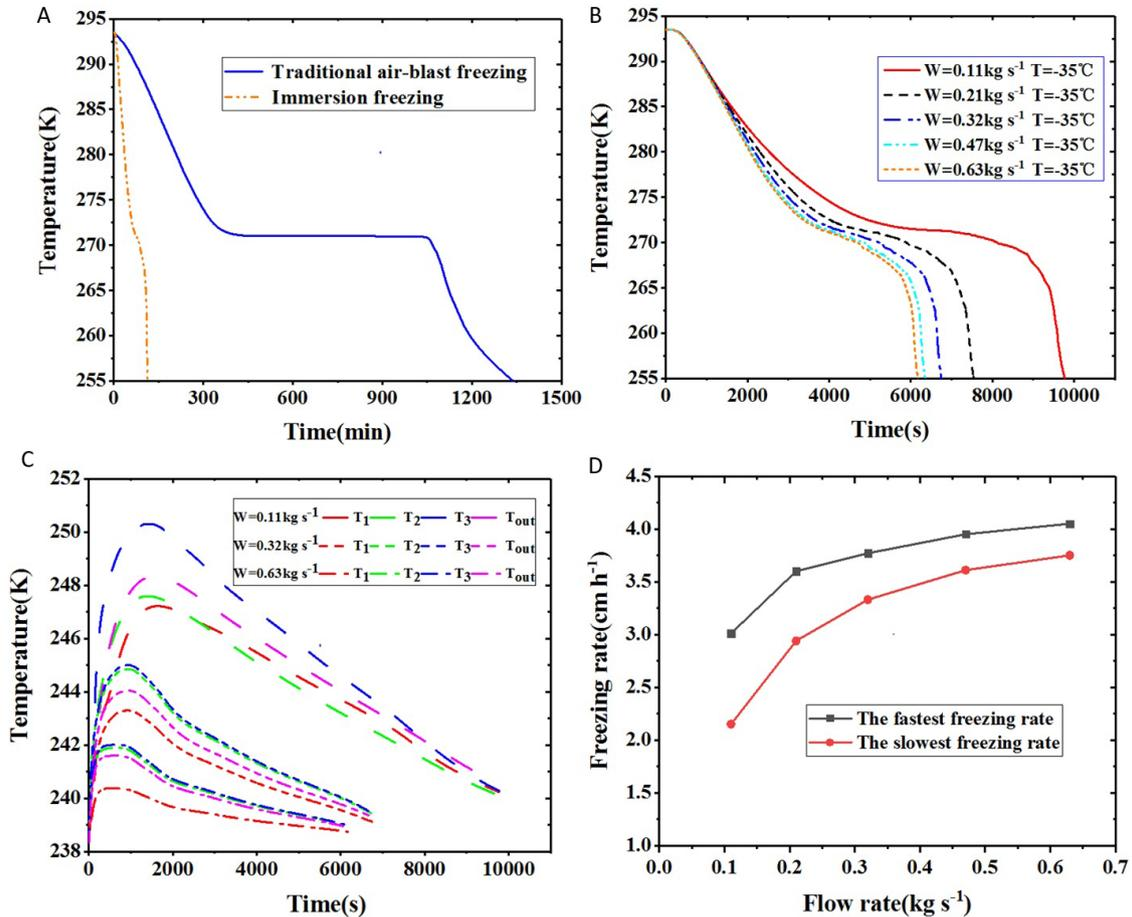
**Figure 4.** Variations in temperature of food at different freezing treatments (A), variation in the temperature of food at different liquid flow rates (B), temperature variations of the refrigerant liquid at different liquid flow rates (C), freezing rate of food at different liquid flow rates (D).
