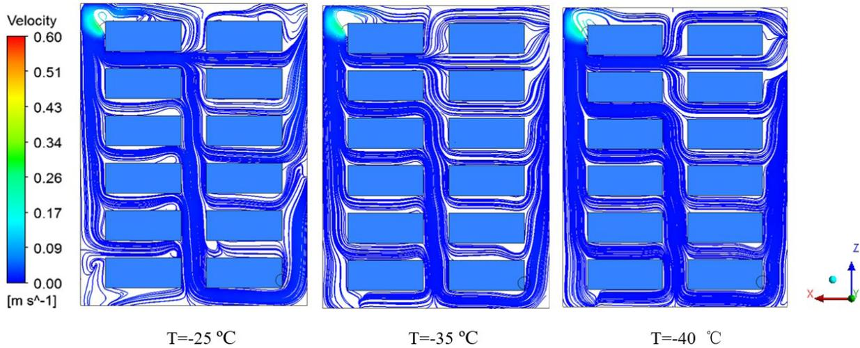
Figure 5. Velocity streamlines in the freezing tank at different liquid temperatures.
