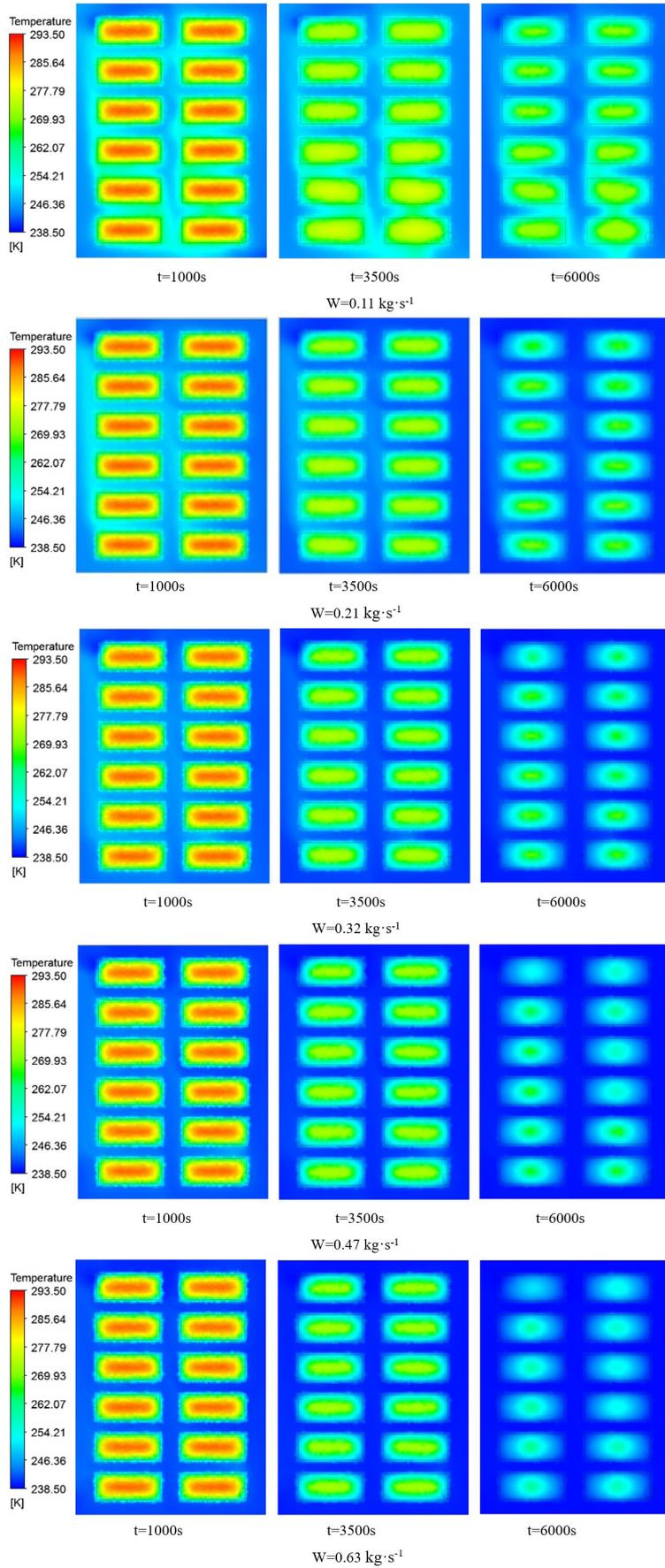
Figure 3. Temperature profiles of the freezing tank at different liquid inlet flow rates.
