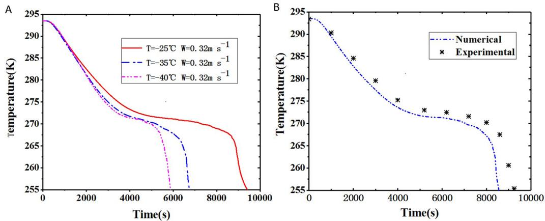
Figure 6. Variations in the temperature of food at different liquid temperature (A), temperature curves of food during the freezing process (B).
