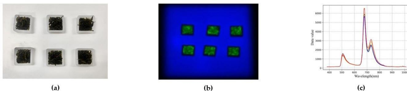
**Figure 1.** Collection of black tea samples image by fluorescence hyperspectral imaging system. (a) six black tea samples on each whiteboard; (b) fluorescence hyperspectral image of samples; (c) fluorescence hyperspectral data of samples.
