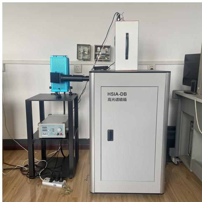
**Figure 2.** Fluorescence hyperspectral system.
