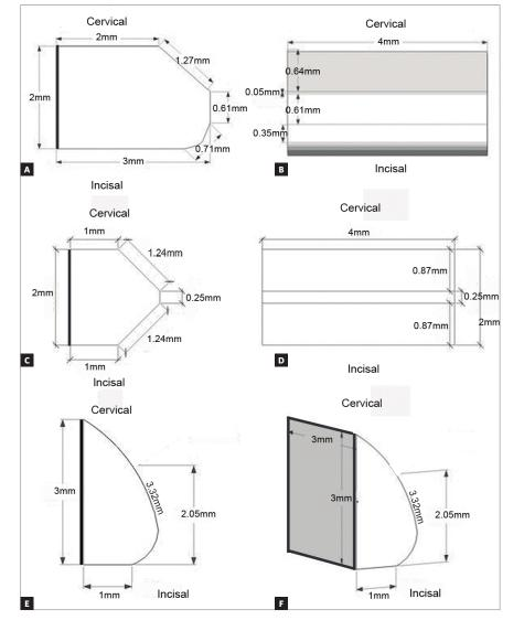
Figure 1 - Attachment 1 in lateral view (A) and frontal view (B). Attachment 2 in lateral view (C) and frontal view (D). Attachment 3 in lateral view (E) and isometric view (F).
