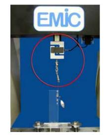
FIGURA 2 - Acrylic plate perpendicularly positioned to the ground on the grip of the testing machine.
