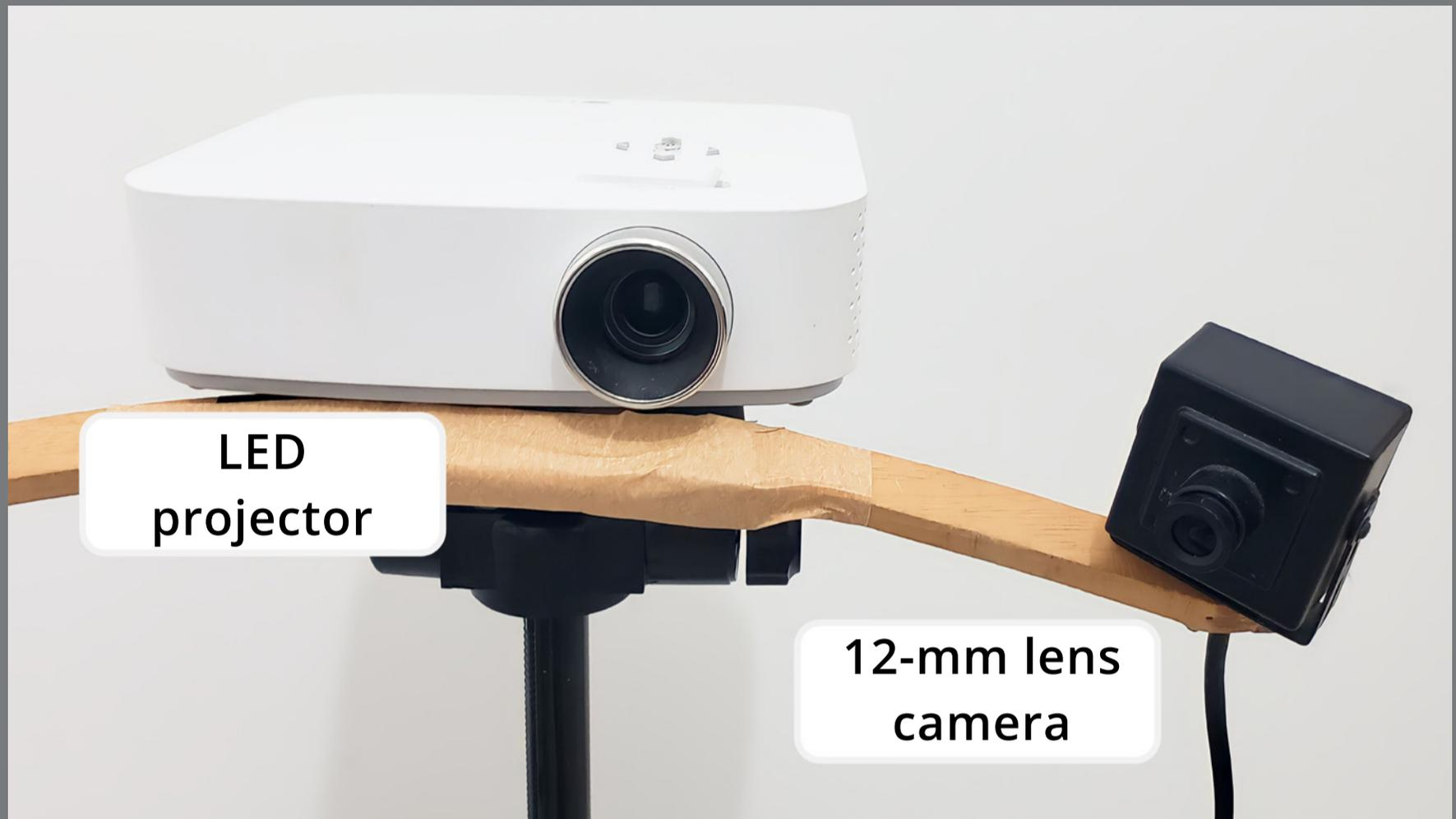
**Figure 1:** Home-built, cost-effective structured light scanning setup. Light patterns were projected using a LED projector (PF50KS, LG Corporation, Seoul, South Korea), and images were captured by a high-resolution 12-mm lens camera (ELP 1080P HD, Ailipu Technology Co., Ltd, Shenzhen, China).
