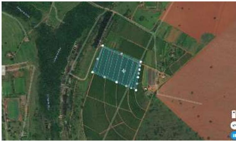
FIGURE 4. Polygon example of the autonomous flight path illustrated in DroneDeploy software.
