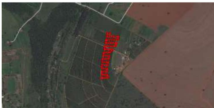
FIGURE 5. Alignment of the photos for image processing and model generation (for volume estimation) in the PIX4D Mapper software.
