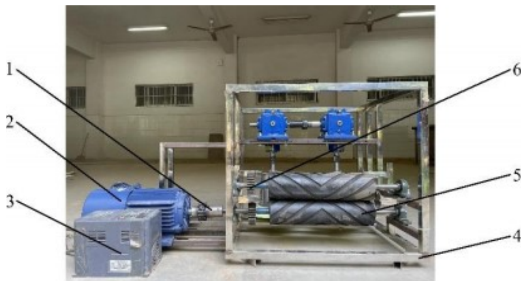
1. Shaft coupling 2. Motor 3. Frequency Converter 4. Frame 5. Conditioning roll 6. Gears.
