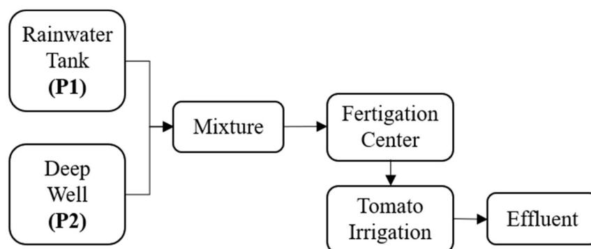
FIGURE 1. Schematic diagram of the water system studied, showing the main collection points in an open cycle: water supply (rainwater tank and deep well), nutrient solution at fertigation center, and effluent solution.
