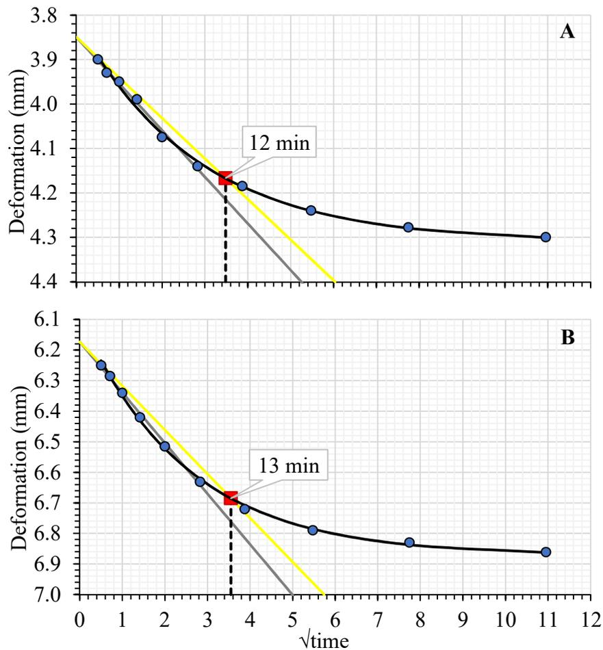
FIGURE 3. Soil compression curve to determine the time required to reach 90% of the maximum deformation for load of 200 (A) 1600 kPa (B), using the square-root of the time method (Taylor, 1948).
