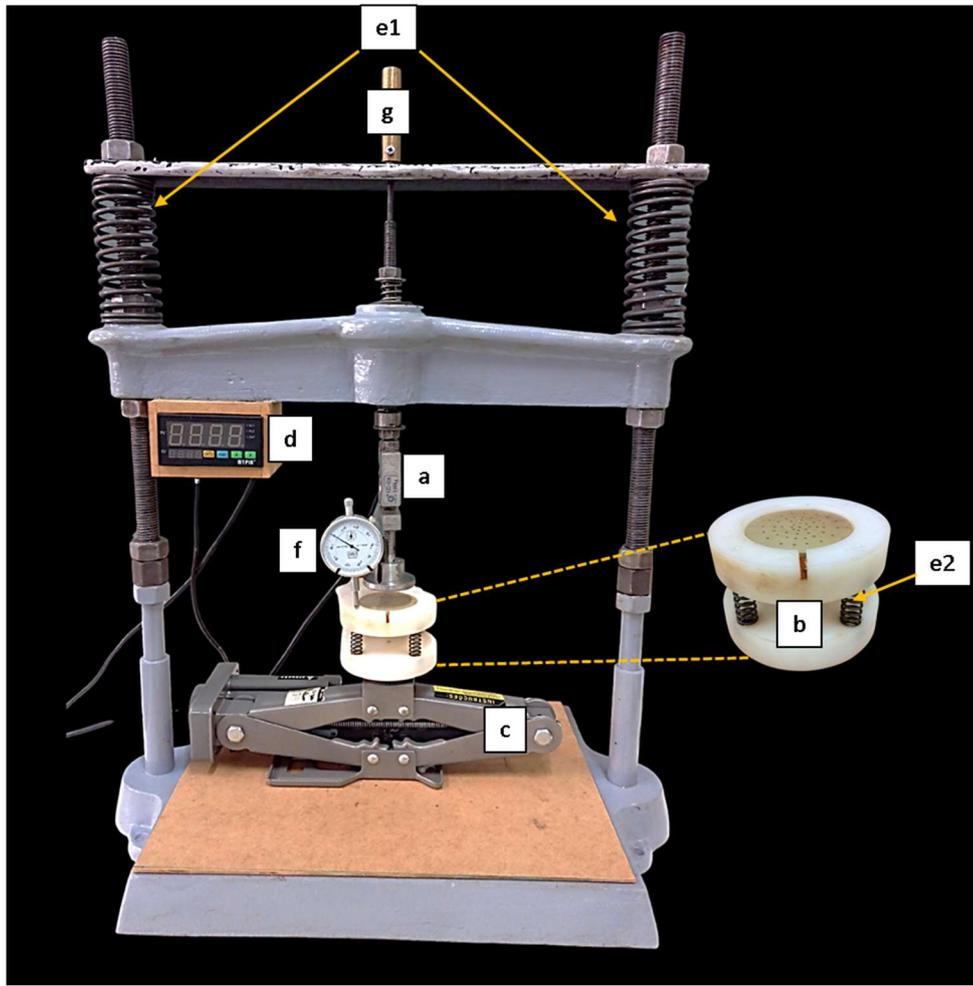
FIGURE 1. Low-cost electro-mechanical press to perform the uniaxial compression test. Components: a – load cell 500 kg; b – compression cell; c – electric jack; d – Digital Weighing Controller Load-cells Indicator; e1 – springs for stabilizing larger loads; e2 – springs for stabilizing smaller loads; f – dial indicator; g – screw for fine load adjustment.
