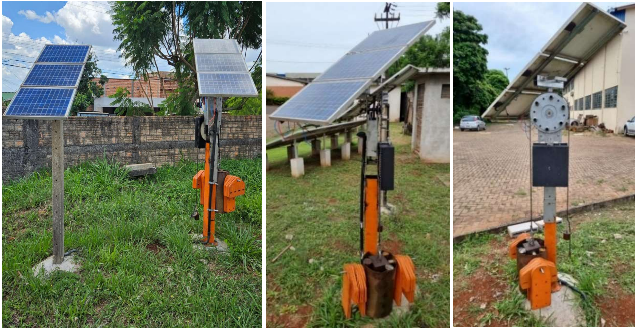
FIGURE 7. P1 - stationary (left) and prototype details for P2 - trackable (right).
