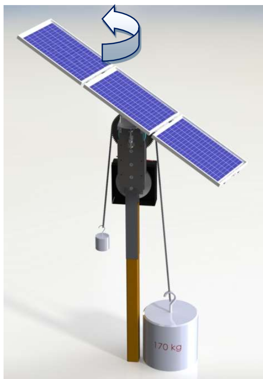
FIGURE 4. Conceptualization of the azimuthal axis tracking prototype.
