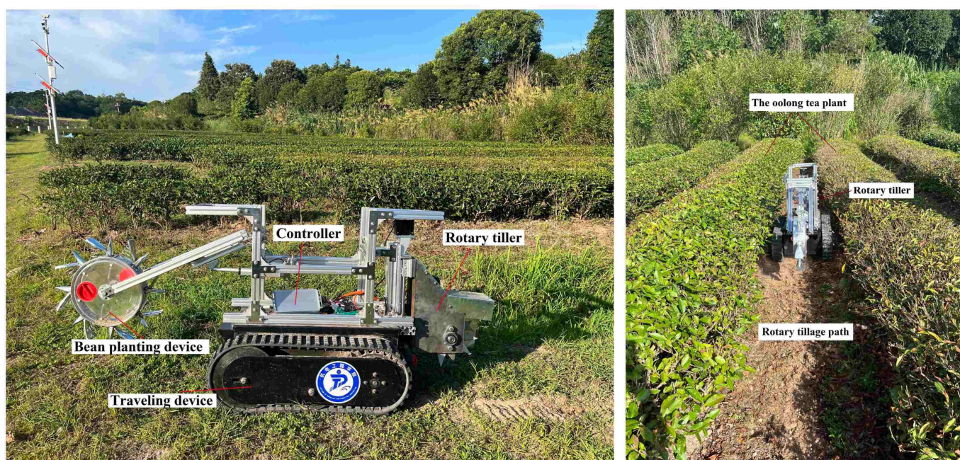
FIGURE 13. Electric Tiller Working Experiment.
