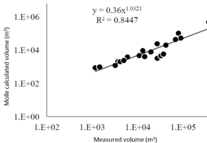
FIGURE 3. Comparative graph for volumes obtained by truncated cone and Molle equation.
