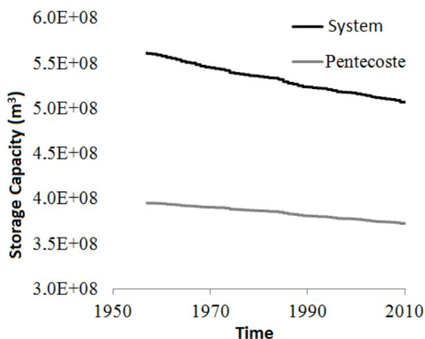
FIGURE 6. Storage capacity decay in Pentecoste weir.
