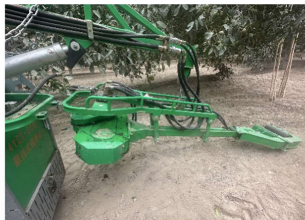
FIGURE 2. Structure of symmetrical eccentric vibration harvesting machine for walnuts.
