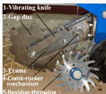
(a) Support cutting anti-clogging device with vibration for no-till seeder
