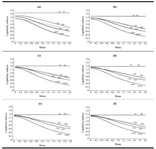
**Figure 3.** Estimates of the capability indices as a function of the process mean (μ), for 5(a), 10 (b), 15 (c), 20 (d), 25 (e) and 30 (f) rational subgroups (m) or sample elements (n).
