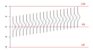
**Figure 2.** Normal distributions with means (μ) equal to 0; 0.1; 0.2; 0.3; 0.4; 0.5; 0.6; 0.7; 0.8; 0.9; 1.0; 1.1; 1.2; 1.3; 1.4; 1.5; 1.6; 1.7; 1.8; 1.9; 2.0 and standard deviation (σ) equal to 1.
