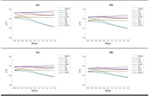
**Figure 6.** Coefficients of variation of the capability indices as a function of the process mean (μ), for 15 (a), 20 (b), 25 (c), 30 (d) rational subgroups (m) or sample elements (n).
