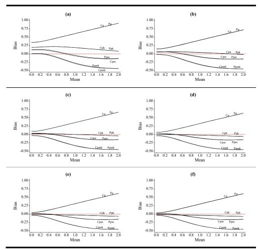
**Figure 4.** Biases of the capability indices as a function of the process mean (μ), for 5 (a), 10 (b), 15 (c), 20 (d), 25 (e) and 30 (f) rational subgroups (m) or sample elements (n).
