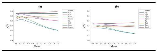
Figure 5. Coefficients of variation of the capability indices as a function of the process mean ( $\mu$ ), for 5 (a) and 10 (b) rational subgroups (m) or sample elements (n).
