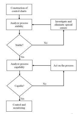
Figure 1. Schematic of Statistical Process Control. Source: Álvarez et al. (2015).
