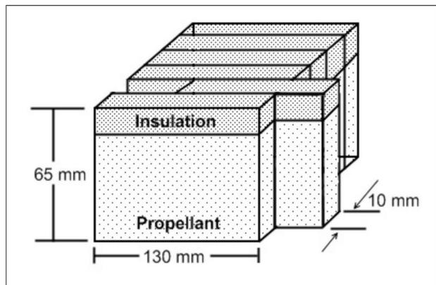
Figure 2: Scheme of the partition of the block of propellant sample.
