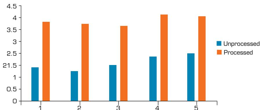
Figure 7. Hybrid composites impact strength vs. composite process.
