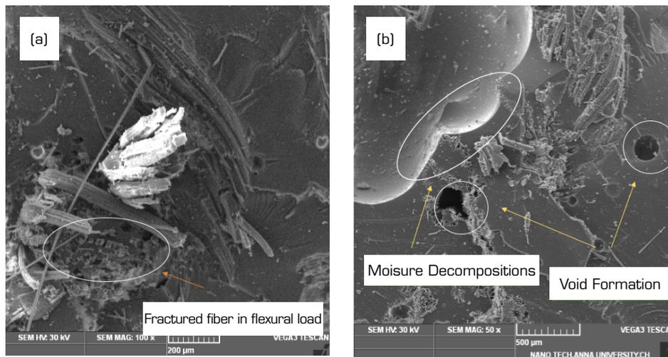
**Figure 12.** Scanning electron microscopy images of composites (a) processed and (b) unprocessed flexural load.
