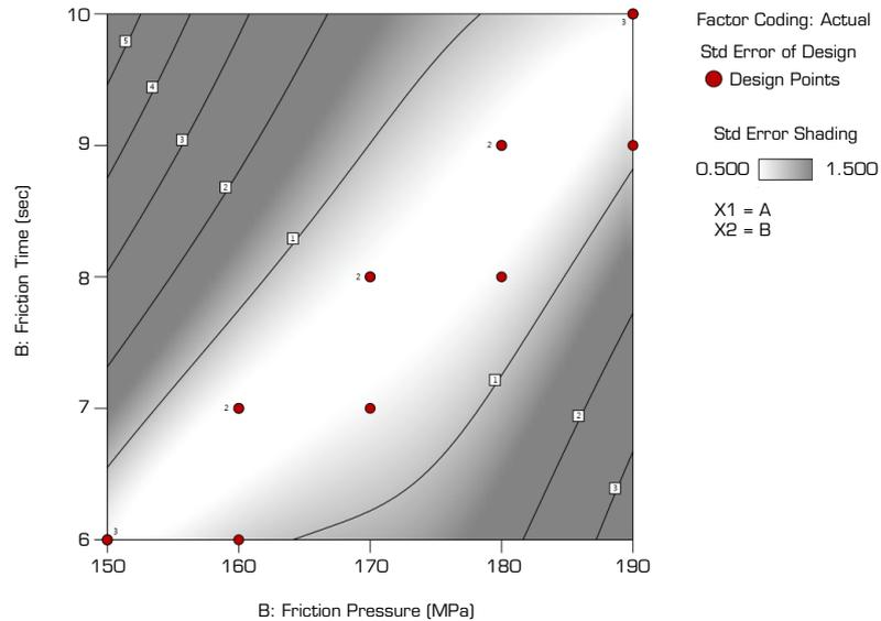
Figure 10. Standard error design in the experimental samples.
