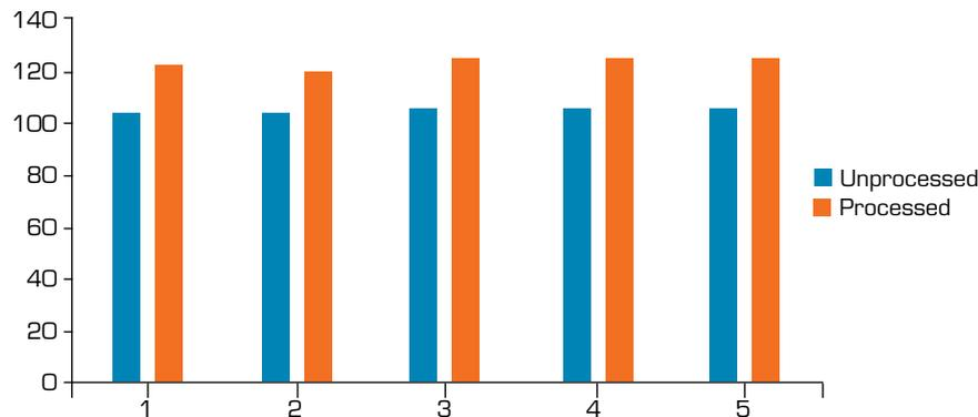
**Figure 5.** Flexural strength vs. composite process results.
