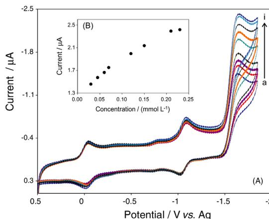
**Figure 6.** (A) Cyclic voltammograms for DMSO containing  $0.05 \text{ mmol L}^{-1}$  TBAP in the presence of  $0.04 \text{ mmol L}^{-1}$  Fe(TPP)Cl, and different concentrations of isoflurane: (a)  $3 \times 10^{-5}$ , (b)  $4.5 \times 10^{-5}$ , (c)  $6 \times 10^{-5}$ , (d)  $7 \times 10^{-5}$ , (e)  $1.2 \times 10^{-4}$ , (f)  $1.5 \times 10^{-4}$  and (g)  $2.1 \times 10^{-4} \text{ mol L}^{-1}$ . (B) Plot of the peak currents as function of concentrations of isoflurane.
