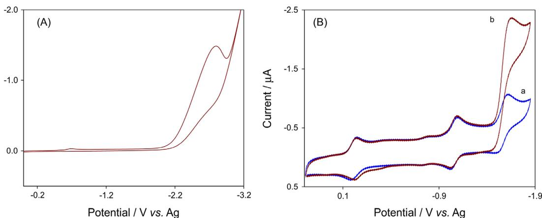
**Figure 3.** (A) Cyclic voltammogram of the DMSO solution containing  $2.1 \times 10^{-4} \text{ mol L}^{-1}$  isoflurane and  $0.05 \text{ M}$  TBAP. (B) Representative cyclic voltammograms of  $0.04 \text{ mmol L}^{-1}$  Fe(TPP)Cl complex (a) in the absence and (b) in the presence of  $2.1 \times 10^{-4} \text{ mol L}^{-1}$  isoflurane in DMSO solution containing  $0.05 \text{ M}$  TBAP. Scan rates were  $100 \text{ mV s}^{-1}$ .
