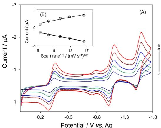
**Figure 2.** (A) Cyclic voltammograms for  $0.04 \text{ mmol L}^{-1}$  Fe(TPP)Cl on a glassy carbon electrode in DMSO solution containing  $0.05 \text{ mol L}^{-1}$  TBAP at scan rates: (a) 25; (b) 50 (c) 100; (d) 150; (e)  $250 \text{ mV s}^{-1}$ . (B) Plots of anodic and cathodic peak currents against (scan rate)<sup>1/2</sup> for both anodic and cathodic peaks for first couple.
