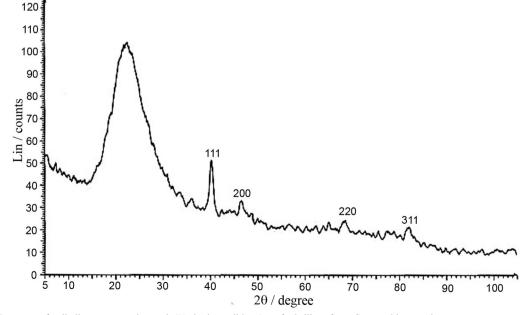
Figure 2. XRD pattern of palladium supported on poly(N-vinylpyrrolidone)-grafted silica after a Sonogashira reaction.
