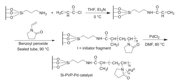
Scheme 1. Preparation of Pd supported on poly(N-vinylpyrrolidone)-grafted silica.
