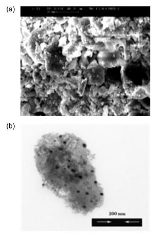
Figure 1. (a) SEM image and (b) TEM image of palladium supported on poly(*N*-vinylpyrrolidone)-grafted silica.<sup>38</sup>
