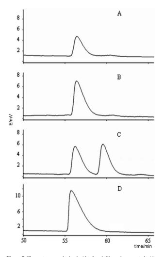
**Figure 2.** Chromatograms obtained with a fused silica column coated with a 1:1-mixture of heptakis-(6-*O*-tert-butyldimethylsilyl-2,3-di-*O*-methyl)- $\beta$ -cyclodextrin and OV-1701 showing the area of elution of grandisol: (A), natural extract, (B), natural extract after treatment with LiAlH<sub>4</sub> (C), synthetic racemic grandisol, (D), synthetic (1*R*, 2*S*)-(+)-grandisol.
