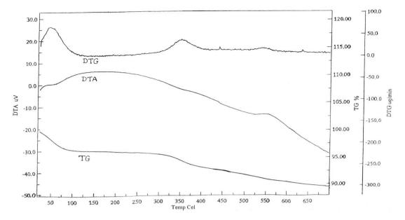
Figure 1. TG-DTG-DTA of silica functionalized sulfonic acid (SiO<sub>2</sub>-SO<sub>3</sub>H).
