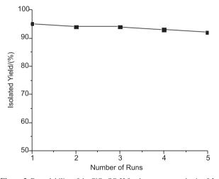
**Figure 2.** Recyclability of the  $SiO_2$ -SO<sub>3</sub>H for the one-pot synthesis of **4c** from 4-chlorobenzaldehyde, urea, 4-fluoroacetophenone and KHSO<sub>4</sub> by stirring in acetonitrile at 80 °C for 10 h.
