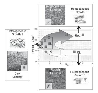
**Figure 8.** Classification of low temperature pyrocarbons: FWHM $_{\rm D}$ , broadening of the Raman D-band vs R $_{\rm A}$ , the Raman anisotropy factor. The arrow indicates the increasing maturation of the gas phase. The three main pyrocarbon-growth-mechanisms are illustrated with their HR-TEM images in high resolution and electron diffraction. Adaptation from Reference 20.
