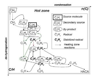
**Figure 5.** Reaction schemes of dehydrogenation and condensation during the cracking of propane for longer and longer residence time in the hot zone of the furnace; the final step being the HACA process (hydrogen abstraction, condensation of acetylene). Adaptation from Reference 20.
