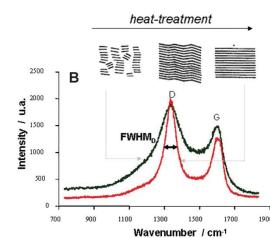
**Figure 7.** Polarised Raman spectroscopy: A)  $R_A$ , Raman anisotropy factor, is the integrated intensity measured under cross- polars divided by the intensity with the polarizer alone; B) Broadening of the D-band as a function of defects' density. Adaptation from Reference 20.
