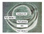
**Figure 4.** Nuclear fuel particle (diameter: 400 to 600  $\mu$ m) coated with a multilayer of porous pyrocarbon (PyC buffer), dense pyrocarbons (dense PyC) and silicon carbide (SiC).
