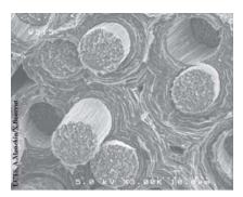
**Figure 2.** Carbon/carbon composite:carbon fiber-reinforced pyrocarbon (SEM picture of a failure surface).
