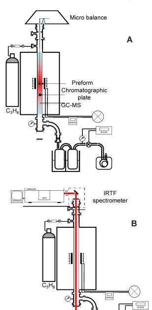
**Figure 6.** Experimental instrumented reactor to establish deposit kinetics (A) and existence diagram of deposit structures versus gaseous compositions (B). Adaptation from Reference 20.
