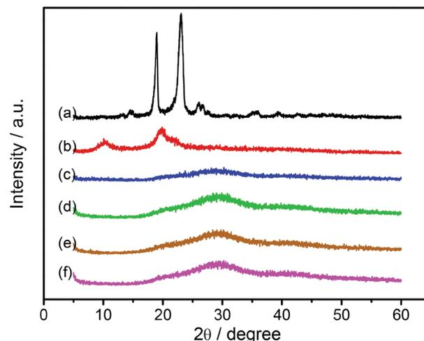
**Figure 10.** X-ray diffractograms of the samples: (a) PEO powder, (b) Ch powder; (c) Ch-PEO electrospun film, (d) Ch-PEO/AO, (e) Ch-PEO/E and (f) Ch-PEO/F (electrospun films).
