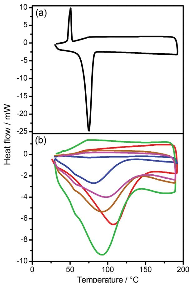
**Figure 9.** Differential scanning calorimetry curves obtained for the materials: (a) PEO powder; (b) (—) Ch powder; (—) Ch-PEO electrospun film; (—) Ch-PEO/AO electrospun film; (—) Ch-PEO/E electrospun film; (—) Ch-PEO/F electrospun film.
