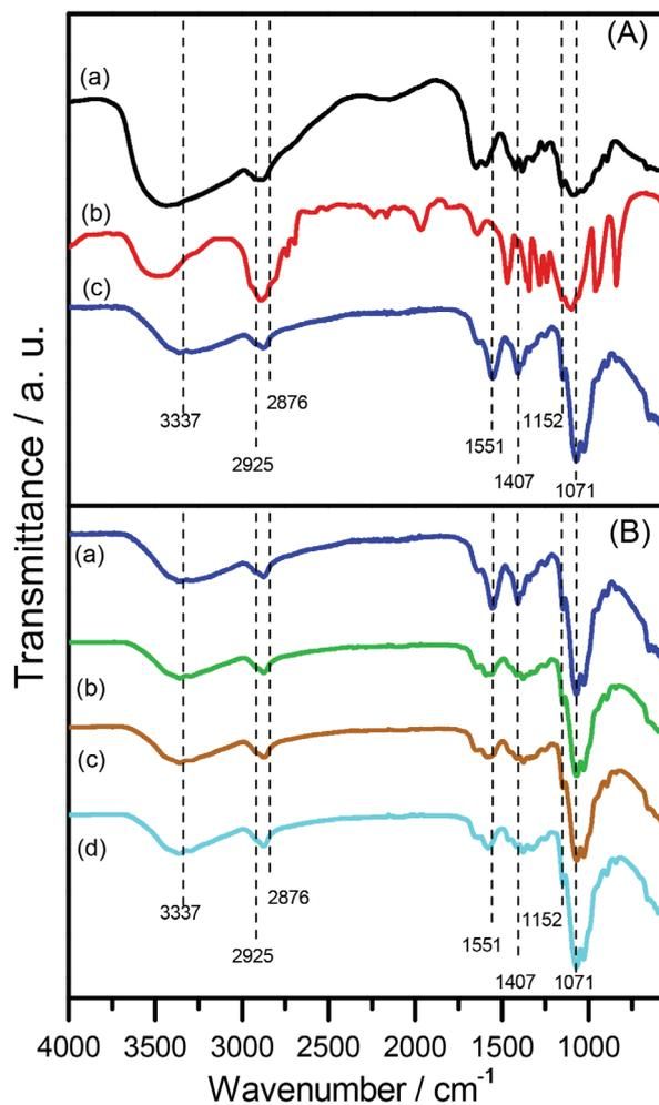
**Figure 7.** (A) FTIR spectra of (a) Ch and (b) PEO powder samples; and of (c) Ch-PEO electrospun film. (B) FTIR spectra of electrospun films: (a) Ch-PEO, (b) Ch-PEO/AO, (c) Ch-PEO/E, and (d) Ch-PEO/F.
