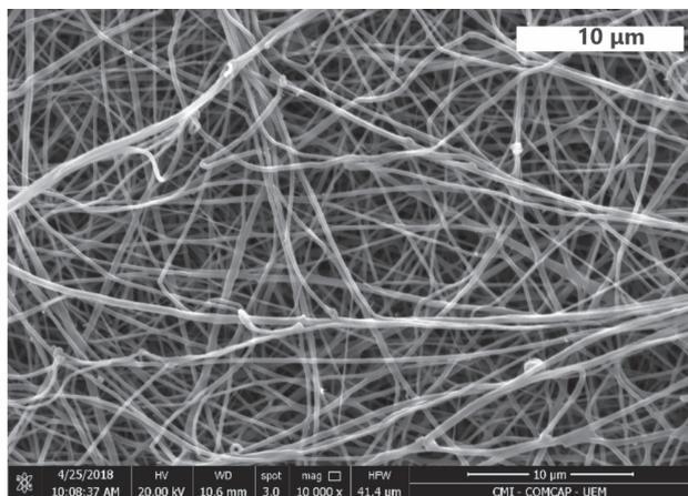
**Figure 2.** SEM micrograph (10,000 $\times$ ) of Ch-PEO electrospun fibers produced from the 2% m/v concentration solution and 90:10% m/m (Ch:PEO) at a distance of 18 cm and an applied voltage of 18 kV.
