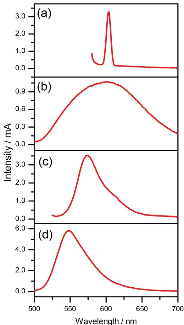
**Figure 6.** Fluorescence spectra (emission) of the (a) Ch-PEO/AO ( $\lambda_{exc} = 570$  nm); (b) Ch-PEO/AO ( $\lambda_{exc} = 473$  nm); (c) Ch-PEO/E and (d) Ch-PEO/F.
