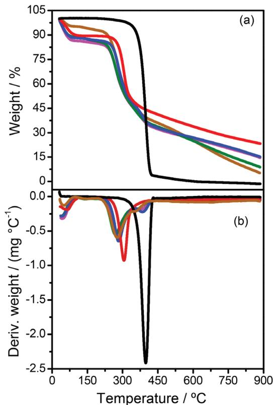
**Figure 8.** (a) Thermogravimetric curves and (b) derived from the thermogravimetric curves of the obtained polymers: (—) PEO powder; (—) Ch powder; (—) Ch-PEO electrospun film; (—) Ch-PEO/AO electrospun film; (—) Ch-PEO/E electrospun film; (—) Ch-PEO/F electrospun film.
