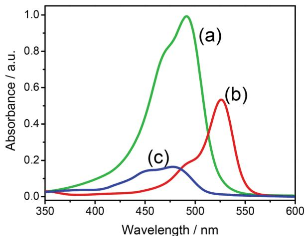
**Figure 4.** Absorption spectra of (a) acridine orange, (b) erythrosine, and (c) sodium fluorescein dyes at 0.001% m/v in aqueous solution.
