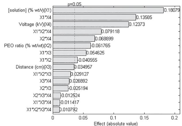
**Figure 1.** Pareto chart showing the effects of solution concentration (X1), Ch:PEO ratio (X2), the distance between the needle and the collector (X3) and applied voltage (X4) on the average diameter of Ch-PEO fibers.
