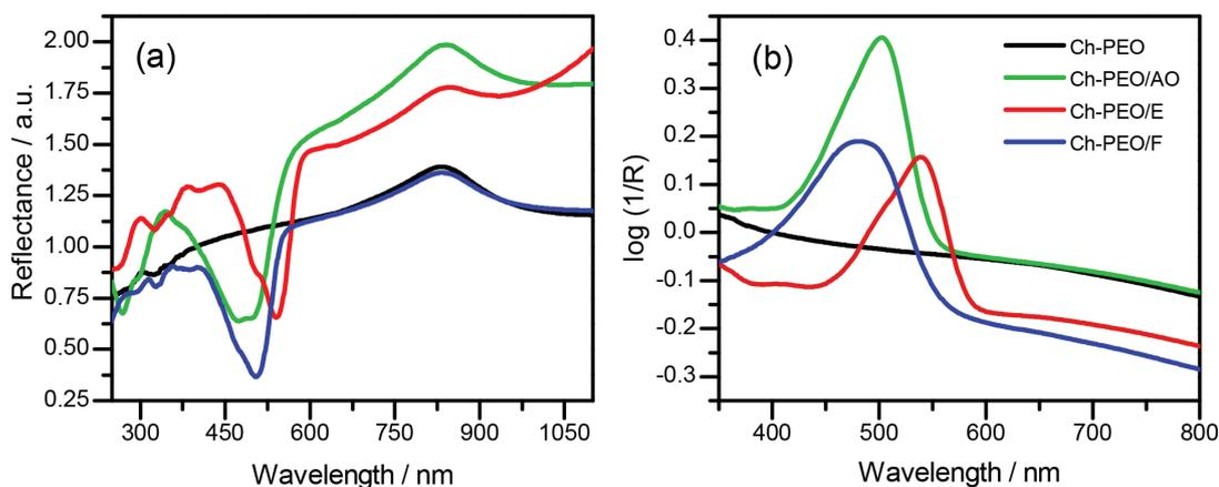
**Figure 5.** (a) Reflectance spectra and (b) absorbance (log (1/R)) of electrospun dye-impregnated films in visible spectra: (—) Ch-PEO without dyes, (—) Ch-PEO/AO, (—) Ch-PEO/E and (—) Ch-PEO/F.
