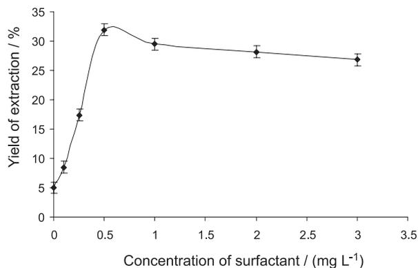
**Figure 1.** Effect of surfactant concentration on yield extraction.
