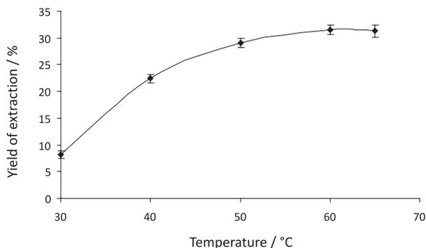
**Figure 3.** Effect of temperature on yield extraction.
