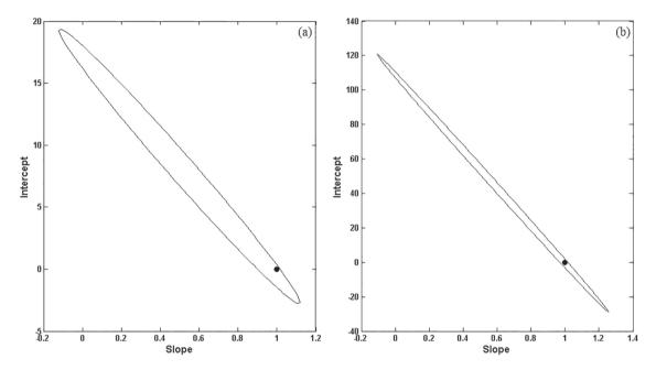
Figure 4. Elliptical joint confidence regions at 95% for the slope and intercept of the regression of predicted n-3 (a) and n-6 (b) against reference values by using ordinary least squares.
