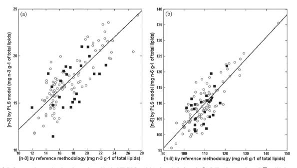
Figure 3. Reference values against the values estimated by the NIR/PLS model (a) for n-3; (b) for n-6. ( $\bigcirc$ ) Calibration samples and ( $\blacksquare$ ) validation samples.
