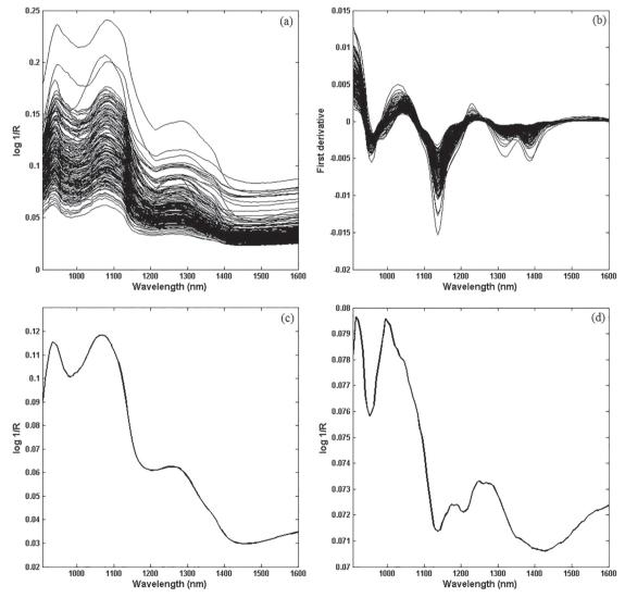
Figure 2. NIR spectra of fillets of Nile tilapia samples. (a) Raw spectra; (b) spectra after first derivative; (c) Nile tilapia without package; (d) package.
