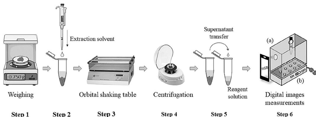
**Figure 1.** Steps involved in the SAs extraction and pre-concentration procedure in bovine meat samples. (a) Bottomless polystyrene box (height: 11 cm; width: 8 cm; depth 14 cm); (b) emergency exit LED light.
