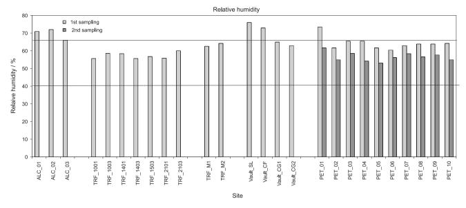
Figure 2. Relative humidity measured for all environments. Lines represent the minimum and maximum relative humidity (40 and 65%, respectively) suggested by Brazilian guidelines.
