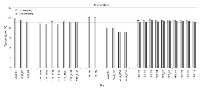
Figure 1. Temperature measured for all environments. Lines represent the minimum and maximum temperatures (23 and 26 °C, respectively) suggested by Brazilian guidelines.
